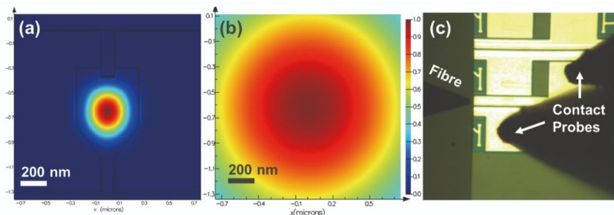
*Figure 5. (a-b) Modal cross-sections of a nano-ridge waveguide and a 2.0 μm focused beam, using a linear colour scale. (c) Top view of measurement setup with cleaved facet and lensed fibre. For more details, see C. I. Ozdemir et al. Dec. 2020, pp. 1–4, doi: 10.1109/ECOC48923.2020.9333310*
