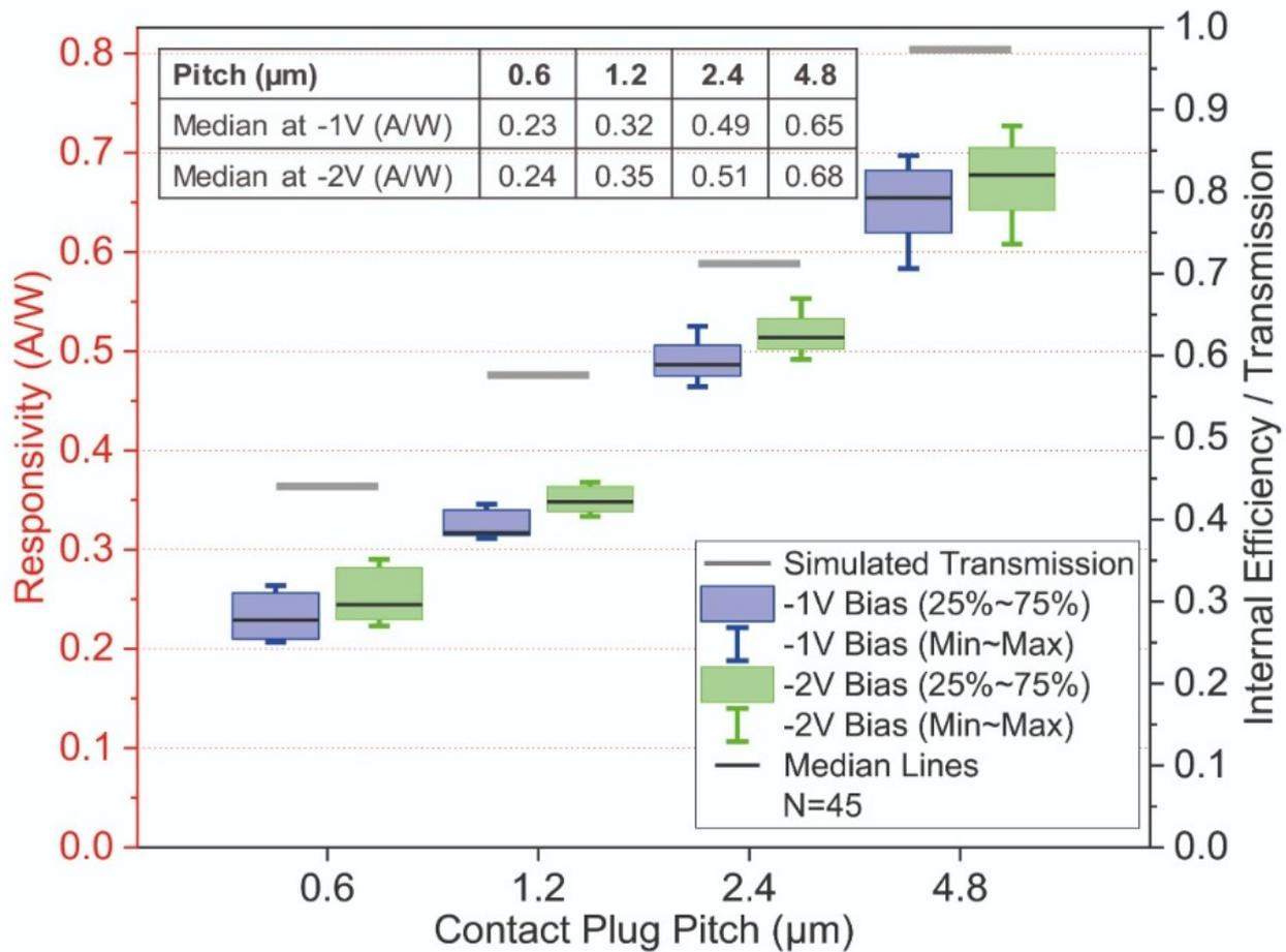
Figure 7. Responsivity distributions for different biases and p-contact plug pitches. Simulated transmission values for different p-contact plug pitches, scaled to right vertical axis. (Inset) Table of median responsivity values. For more details, see C. I. Ozdemir et al. Dec. 2020, pp. 1–4, doi: 10.1109/ECOC48923.2020.9333310
