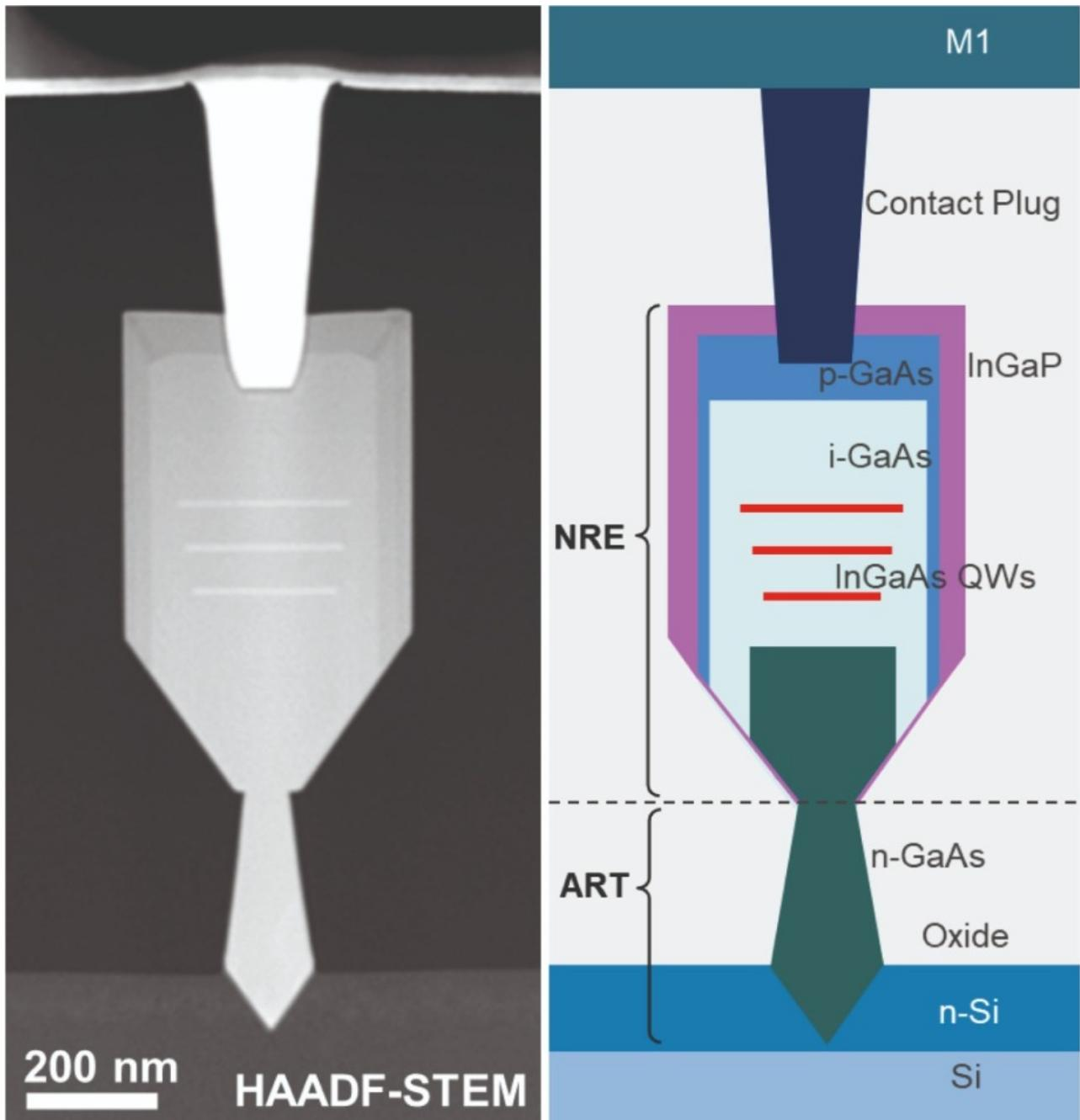
Figure 3. (Right) High-angle annular dark-field scanning transmission electron microscopy (HAADF-STEM) cross-sectional image of GaAs nano-ridge with three InGaAs quantum wells. (Far right) Description of the nano-ridge cross-section. For more details, see C. I. Ozdemir et al. Dec. 2020, pp. 1–4, doi: 10.1109/ECOC48923.2020.9333310
