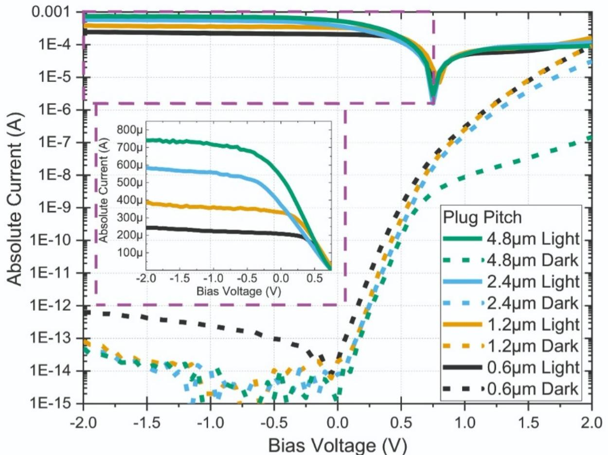
Figure 6. Dark and light measurements of current-voltage (*I-V*) characteristics of devices with different *p*-contact plug pitches, (inset) light *I-V* zoom in at linear scale. For more details, see C. I. Ozdemir et al. Dec. 2020, pp. 1–4, doi: 10.1109/ECOC48923.2020.9333310
