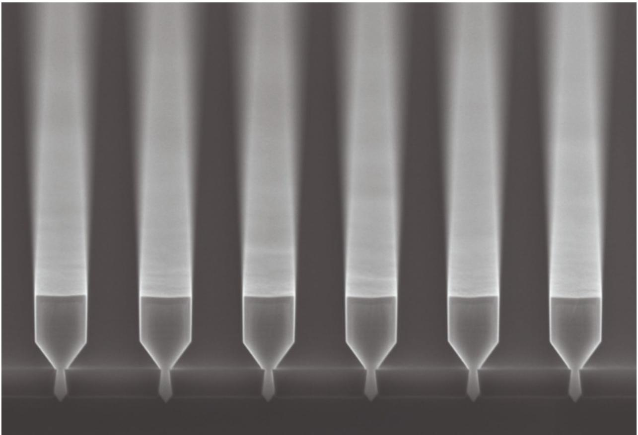
*Figure 1. Tilted scanning electron microscopy (SEM) image of III-V nano-ridges grown on silicon.*
