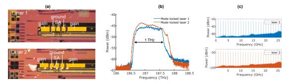
Fig. 1. Overview of the III-V-on-silicon mode-locked lasers. (a) Micrographs of both III-V-on-silicon mode-locked lasers. (b) Optical spectra of both lasers measured with 50 pm resolution. (c) RF spectra of the III-V-on-silicon mode-locked lasers, illustrating stable mode-locking.
