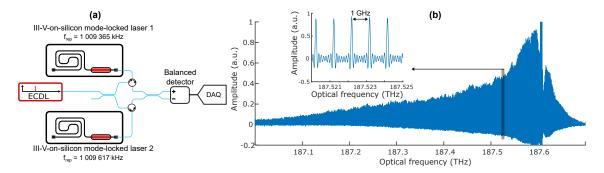
Fig. 2. (a) Schematic layout of the dual-comb interferometer. (b) Dual-comb spectrum of two onchip mode-locked lasers with approximately 700 resolved comb lines, with a line spacing of 1 GHz (inset).
