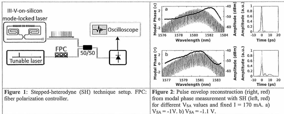
**Figure 1:** Stepped-heterodyne (SH) technique setup. FPC: fiber polarization controller.
