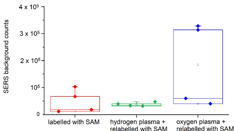
**Figure 2.** SERS background counts integrated between 500 and 1500  $\text{cm}^{-1}$  for the samples labeled with the SAM (red), cleaned with hydrogen plasma and then relabeled with the SAM (green) or cleaned with oxygen plasma and relabeled with the SAM (blue). The points represent the averaged values on individual samples, whereas the box plot represents the statistical distribution of the points.
