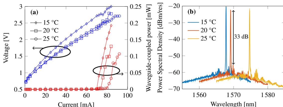
Fig. 2: Basic characterization of the device. **(a)** V-I and L-I curves. **(b)** Measured spectra above threshold.
