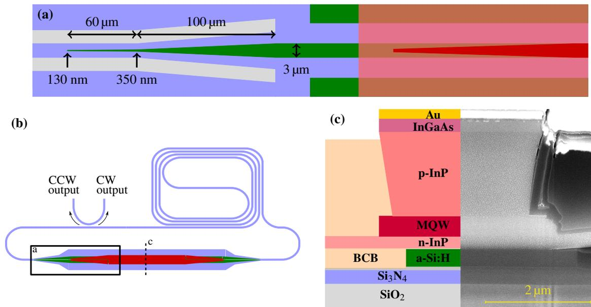
Fig. 1: Schematic layout of the laser cavity and the adiabatic coupling scheme. **(a)** Linear tapering structure. **(b)** Ring laser cavity design. The dashed line indicates the location of the cross-section. **(c)** Schematic drawing of the material stack (left) and SEM image of a cross-section of the device at the center of the amplifier section (right).
