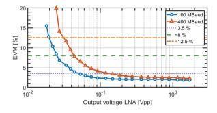
Fig. 13. rms-EVM as a function of the  $V_{out,pp}$  of the LNA.
