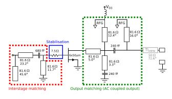
Fig. 5. Amplifier stage 3.
