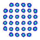
Fig. 16. 4 GBd at 27.5 GHz (5.8% rms-EVM) – 21 km SSMF.
