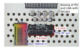
Fig. 7. Narrowband photoreceiver assembly.
