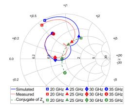
Fig. 9.  $S_{11}$  shown on the Smith chart for a 50  $\Omega$  reference.
