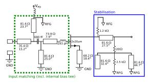
Fig. 3. Amplifier stage 1 (RFG: RF ground).
