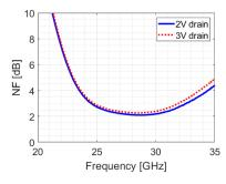
Fig. 10. Simulated noise figure for 2 and 3 V drain supply.
