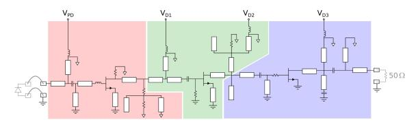
Fig. 6. Overall schematic of the 3-stage near-mmWave low noise amplifier.
