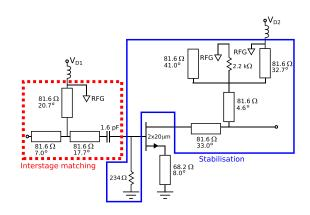
Fig. 4. Amplifier stage 2.
