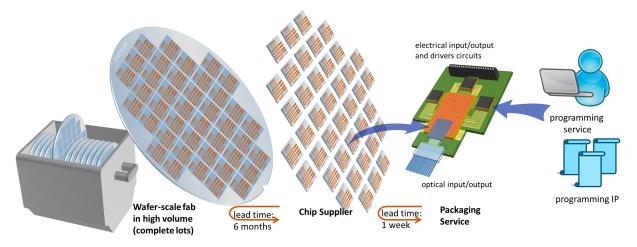
Fig. 2. Generic programmable PICs have a different manufacturing and supply model than ASPICs. They can be fabricated in larger volumes, and supplied off-the-shelf at short notice. Around these chips a new ecosystem of packaging and programming services can evolve.
