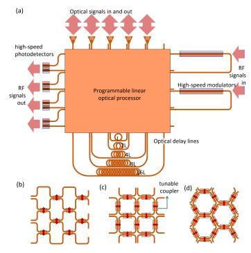
Fig. 1. Conceptual generic programmable photonic circuit. (a) A linear optical processor connects the optical inputs and outputs with active elements such as modulators and photodetectors. The linear circuit can have either (b) a feed-forward architecture of coupled Mach-Zehnder interferometers [2]–[4], or (c-d) a network with rectangular [5] or hexagonal loops. [6]
