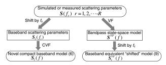
**Fig. 4.** Flow chart of the CVF modeling approach (left branch) and the one presented in Ref. [12] (right branch).
