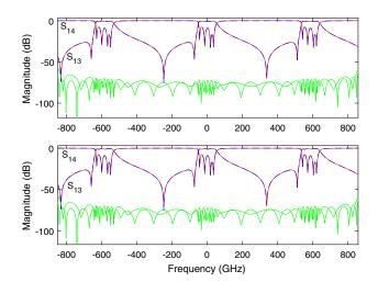
**Fig. 14.** Example 7.B. The accuracy of the VF-based Model (9) (top) built via the technique in Ref. [12] with 42 poles and the CVF Model (6) (bottom) built via the newly proposed technique with 21 poles; the red solid lines represent the simulated scattering parameters, and the blue dashed lines represent the models, while the green lines are the magnitude of the error between the two.
