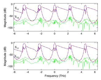
**Fig. 8.** Example 7.A. The accuracy of the VF-based Model (9) (top) built via the technique in Ref. [12] with 108 poles and the CVF Model (6) (bottom) built via the newly proposed technique with 54 poles; the red solid lines represent the simulated scattering parameters, the blue dashed lines represent the models, while the green lines are the magnitude of the error between the two.
