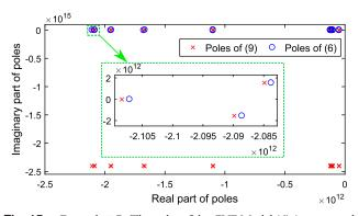
**Fig. 15.** Example 7.B. The poles of the CVF Model (6) (represented by circles) and the Model (9) from the VF-based technique in Ref. [12] (represented by crosses).
