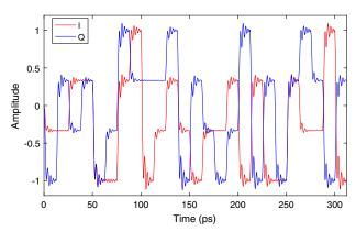
**Fig. 10.** Example 7.A. The in-phase part I(t) and quadrature part Q(t) of the 16 QAM input signal.
