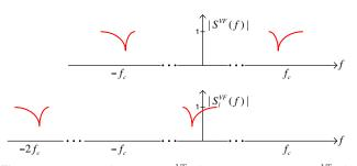
**Fig. 5.** Spectrum of the model  $S^{VF}(f)$  (top) and the model  $S_{l}^{VF}(f)$  represented by Model (9) (bottom).
