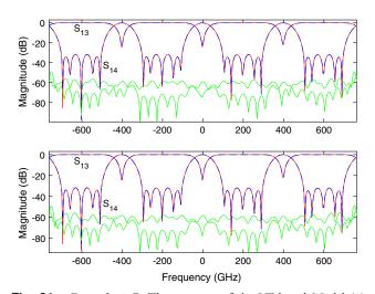
**Fig. 21.** Example 7.C. The accuracy of the VF-based Model (9) (top) built via the technique in Ref. [12] with 68 poles and the new CVF Model (6) with 34 poles (bottom); the red solid lines represent the simulated scattering parameters, and the blue dash lines represent the models, while the green lines show the error between them.
