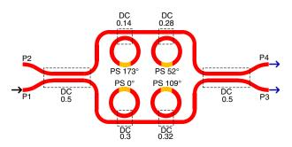
**Fig. 13.** Example 7.B. The schematic circuit of the ring-loaded MZI filter.
