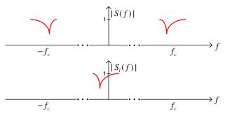
Fig. 2. Spectrum of bandpass systems (top) and the corresponding baseband equivalent systems (bottom).
