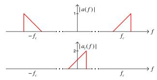
**Fig. 1.** Spectrum of the modulated optical signal (top) and its baseband equivalent signal (bottom).
