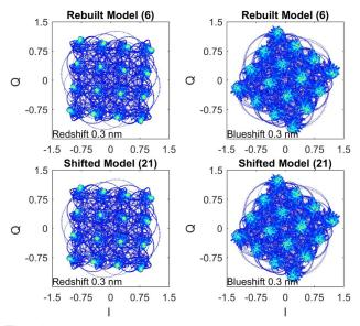
**Fig. 18.** Example 7.B. Constellation diagram of the transmission signal at P3 calculated from the rebuilt CVF Model (6) and the shifted Model (21), when the passband of the filter redshifts and blueshifts by 0.3 nm.
