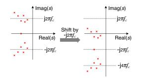
**Fig. 6.** Poles of the model  $S^{VF}(f)$  (left) and the model  $S_l^{VF}(f)$  represented by Model (9) (right).
