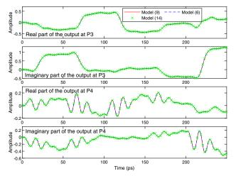
Fig. 16. Example 7.B. The output signals at P3 and P4 obtained from baseband time-domain simulation of Models (6), (9), and (14).
