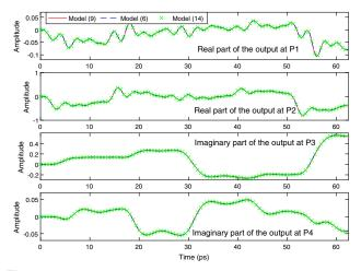
**Fig. 11.** Example 7.A. The output signals at P1, P2, P3, and P4 obtained from baseband time-domain simulations of Models (6), (9), and (14).
