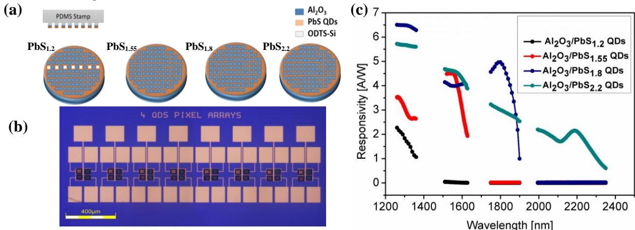
Fig. 1 . (a) A schematic illustration of the transfer-printing process flow from the four  $\text{Al}_2\text{O}_3/\text{QD}$  source substrates using arrayed PDMS stamp, (b) Optical image of a printed array of 8 multi-spectral  $\text{Al}_2\text{O}_3/\text{PbS}$  QD pixels, and (c) Spectral response measured at  $1\mu\text{W}$  power level and 1 V bias
