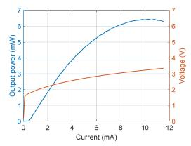
Fig. 7. Output power and voltage as a function of current with power measured without a polarizer.
