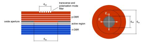
Fig. 2. The oxide-confined VCSEL with a transverse and polarization mode filter etched into the surface. The diameters of the oxide aperture  $(d_{ox})$  and the mode filter  $(d_{ny})$  are indicated and the two orthogonal polarization states  $(E_{\perp} \text{ and } E_{\parallel})$  are defined. Left: side view. Right: top view.
