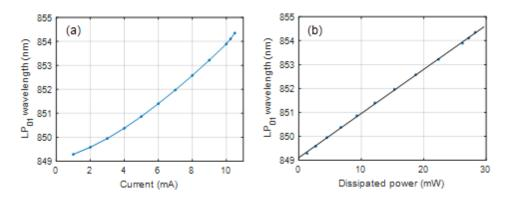
Fig. 10. Wavelength of the fundamental transverse LP01- $E_{\perp}$  mode as a function of a) current and b) dissipated power.
