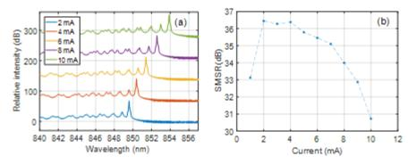
Fig. 9. a) Spectra at different currents from threshold to rollover. b) Higher order transverse mode suppression (side-mode suppression ratio, SMSR) as a function of current.
