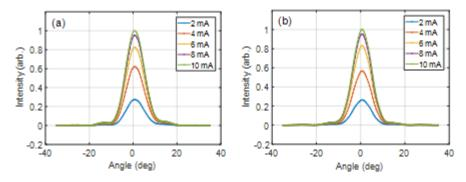
Fig. 11. Measured beam profile along directions perpendicular (a) and parallel (b) to the grating lines at different currents.
