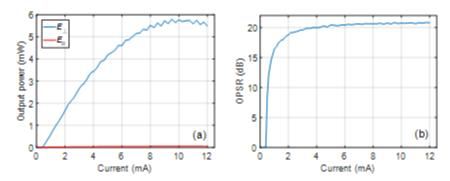
Fig. 8. a) Output power in the two orthogonal polarization states as a function of current, measured with a polarizer between the VCSEL and the photodiode. b) Orthogonal polarization mode suppression (OPSR) as a function of current.
