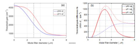
Fig. 3. Dependence of a) threshold gain for the transverse LP01- $E_{\perp}$  and LP11- $E_{\perp}$  modes and b) transverse and polarization mode discrimination (threshold gain differences) on mode filter (grating) diameter. The grating pitch, depth, and fill-factor is 120 nm, 59 nm, and 55%, respectively. The diameter of the oxide aperture is 5  $\mu$ m.
