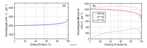
Fig. 4. Dependence of a) threshold gain for the fundamental transverse LP01- $E_{\perp}$  mode and b) transverse and polarization mode discrimination (threshold gain differences) on grating fill-factor. The grating pitch and depth is 120 and 59 nm, respectively, and the oxide aperture and mode filter diameters are 5 and 3  $\mu$ m, respectively.
