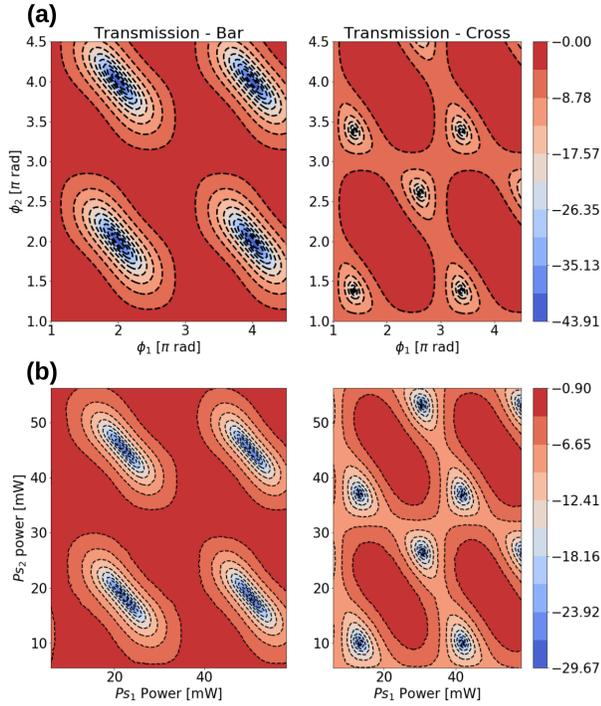
Fig. 2. (a) Simulated result for the two-stage MZI  $2 \times 2$  tunable coupler with power coupling ratio of 27% at  $1.61 \mu\text{m}$ . Power transmission is shown in logarithmic scale. (b) Measured transmission of the fabricated device. We have a strong qualitative agreement between simulation and experiment.
