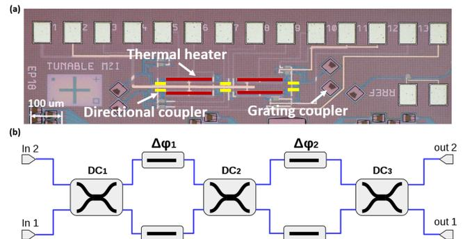
Fig. 1. (a) Microscope picture of the fabricated device.(b) Two-Stage MZI  $2 \times 2$  tunable coupler.
