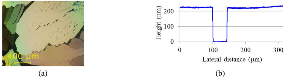
Fig. 2. (a) Polarized light microscopy image. (b) Surface profile of BNA crystals.
