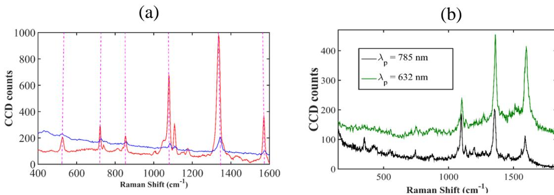
Fig 1. a) The Raman spectra of 4-Nitrophenol measured from a bowtie antenna (blue) and a metal slot waveguide (red) integrated with SiN waveguide. The pink dotted lines represent the Raman modes of NTP. b) The Raman spectra measured from a metal slot waveguide at 785 nm (black) and 632 nm (green) excitation wavelengths.
