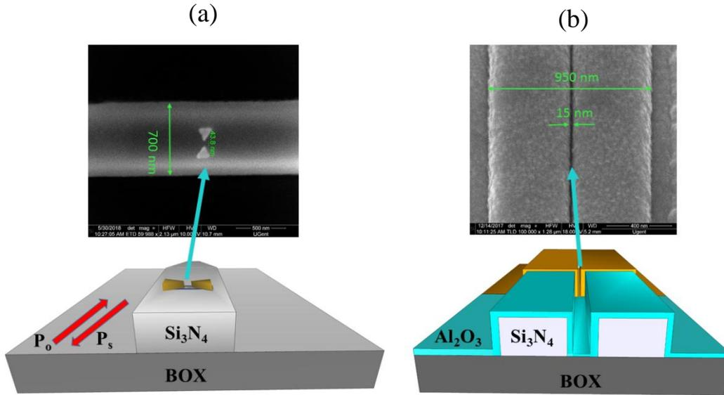
Fig 1. The schematic of the  $\text{Si}_3\text{N}_4$  integrated SERS sensors. a) The bowties antenna integrated a monomode  $\text{Si}_3\text{N}_4$  strip waveguide. b) The plasmonic waveguide interfaced with a monomode AlO clad  $\text{Si}_3\text{N}_4$  slot waveguide. The inset shows the SEM image of the fabricated sensor.
