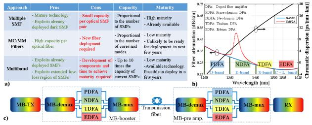
Fig. 1: (a): Comparison among the different solutions; (b): Fiber attenuation and dispersion parameters over the multiband SMF spectrum; (c): Multiband system and bandwidth requirements of the key-components.
