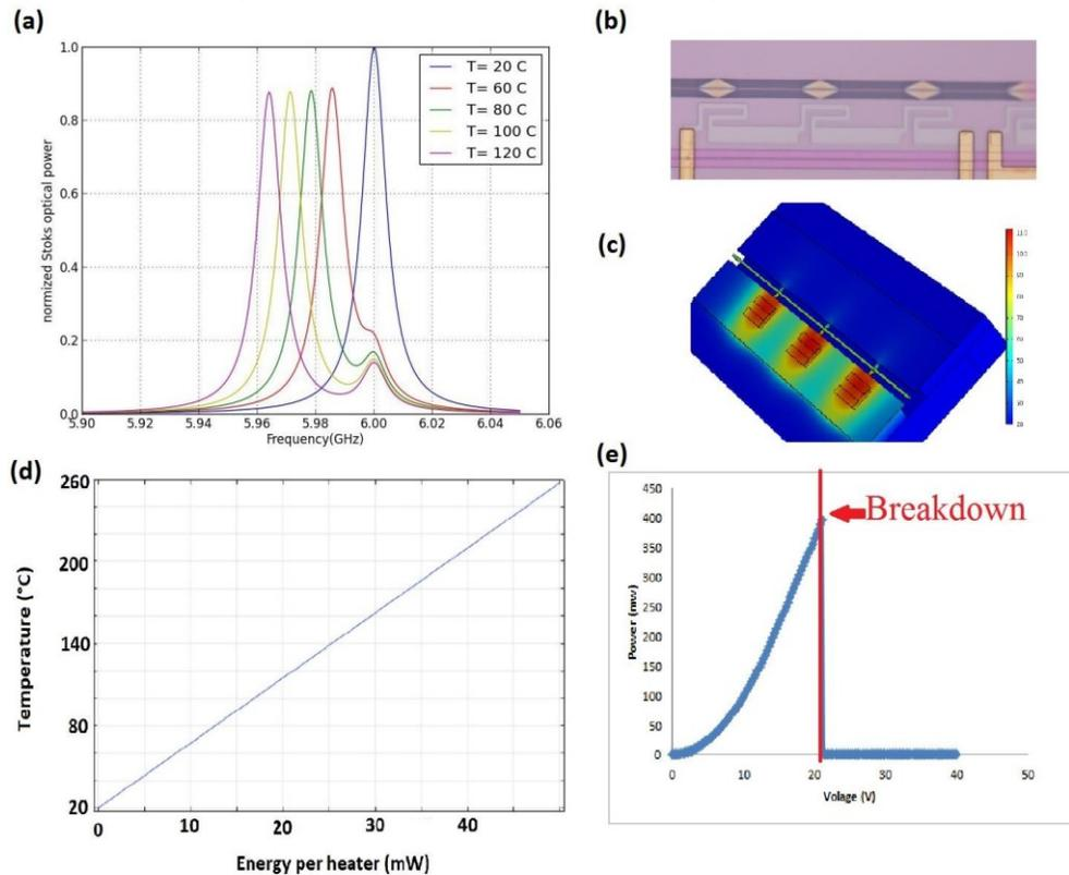
**Figure 2** (a) Free standing WG width mapping: Stokes power vs. heater power (b) Chromium heaters next to the WG anchoring points (c) FEM simulation of thermal transport (d) Free standing WG : temperature vs. heating power per heater (e) under etched Chromium heater characterization
