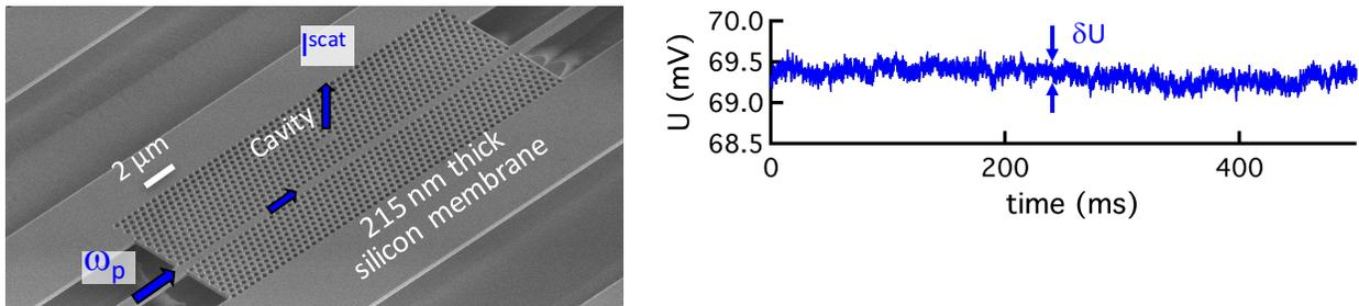
Fig.2. Left: Scanning electron micrograph of the top surface of an integrated L3 PhC cavity. The blue arrows indicate the light path of the pump laser beam at a frequency  $\omega_p$ . Right: Time trace of the photovoltage  $U$  induced by the collected scattered light  $I^{\text{scat}}$  for a detuning between the  $\omega_p$  and the resonance frequency of the cavity, which highlights the presence of a phase noise due to the fundamental thermodynamic fluctuations.
