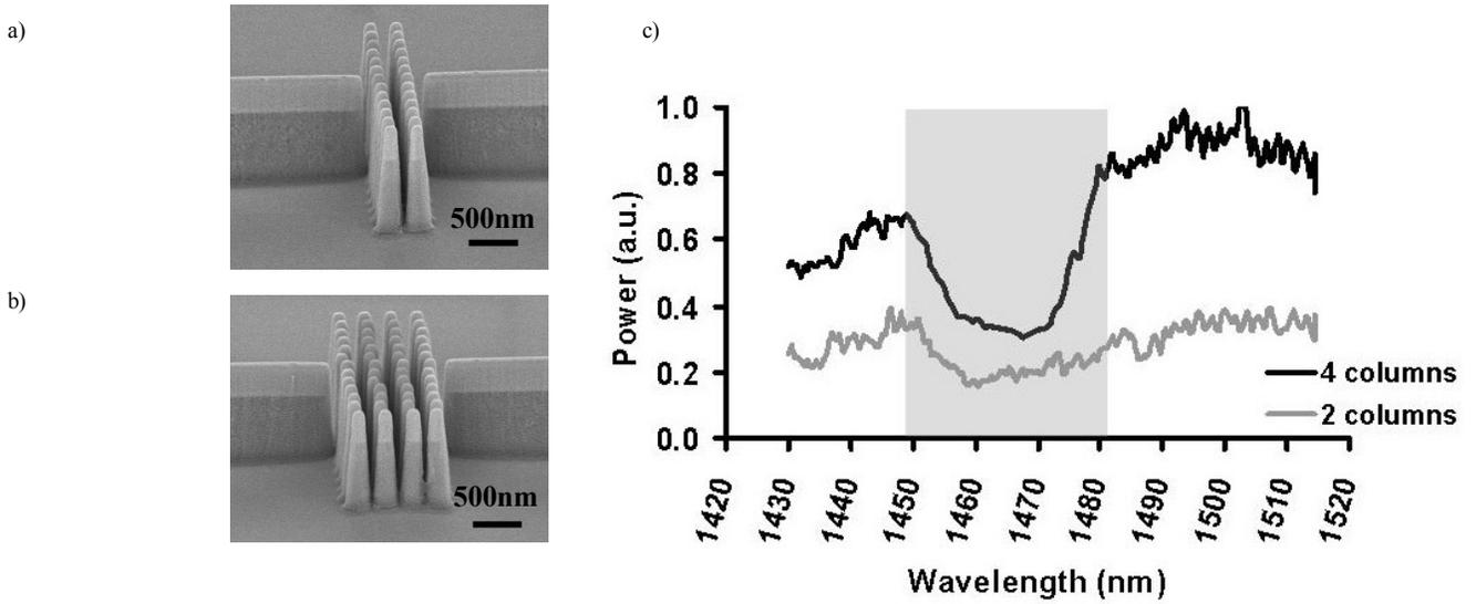
Fig. 2. (a) Scanning Electron Microscope (SEM) image of photonic crystal with 2 columns of dielectric pillars (b) SEM of a photonic crystal with 4 columns of dielectric pillars (c) transmission measurement through the structures in (a) and (b).
