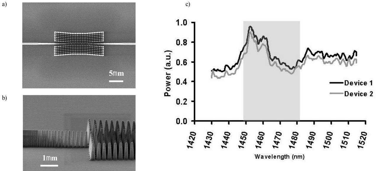
Fig. 3. (a) Top-down SEM image of tapered photonic crystal waveguide (b) Side view SEM of tapered photonic crystal waveguide (c) transmission measurement through the structures in (a) and (b). Two PC waveguides fabricated on the same chip demonstrated similar transmission.
