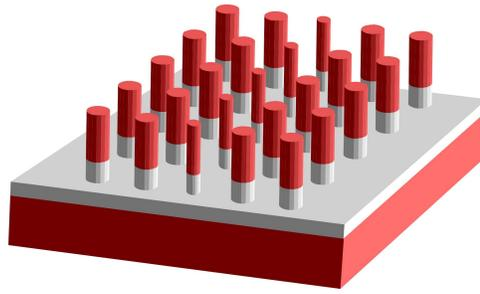
Fig. 1. Schematic representation of a 2D slab photonic crystal waveguide made of cylindrical dielectric pillars.
