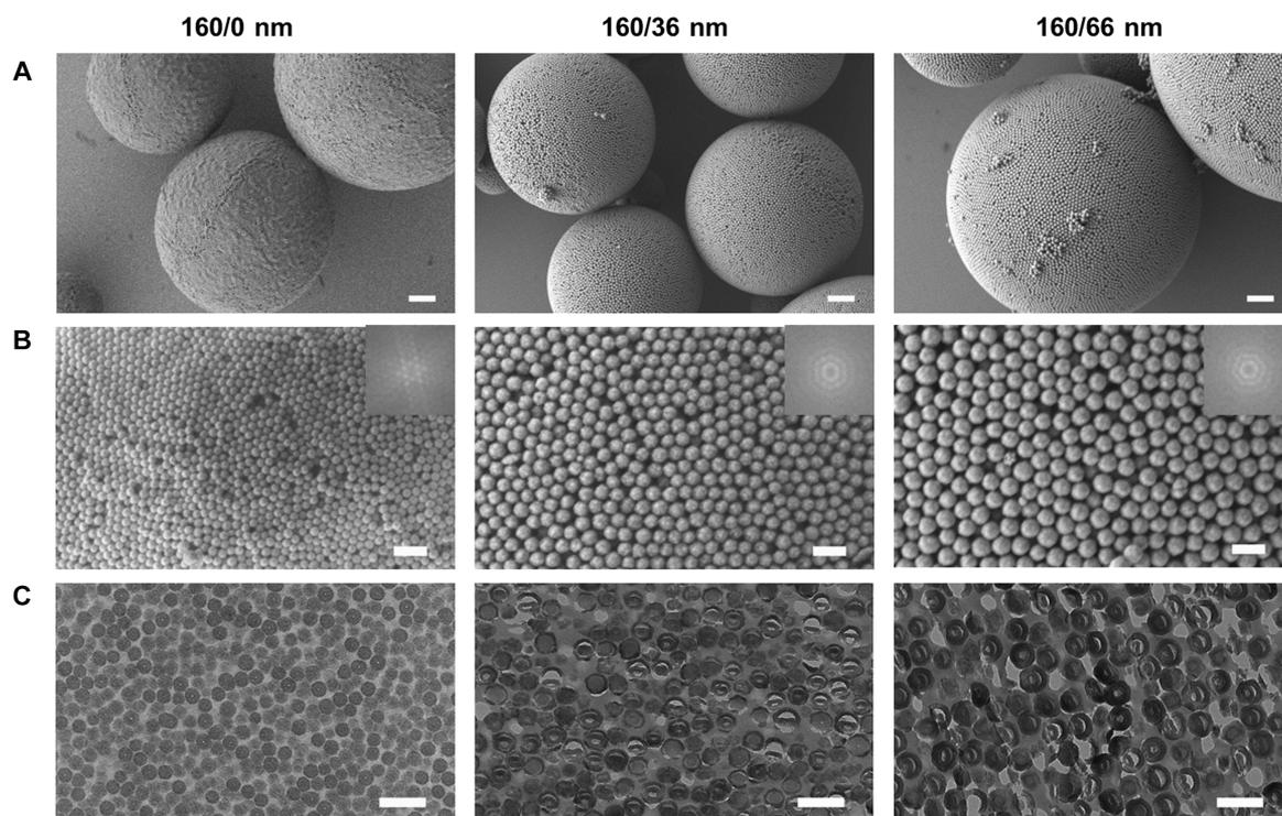
**Fig. 4. Microstructures of supraballs.** Each column represents supraballs made of different sizes of CS-SMNPs. (A) SEM images of whole supraball morphologies. (B) High-resolution SEM images of top surfaces of supraballs. (C) Cross-sectional TEM images of the inner structure of supraballs. Scale bars, 2  $\mu\text{m}$  (A), 500 nm (B), and 500 nm (C).
