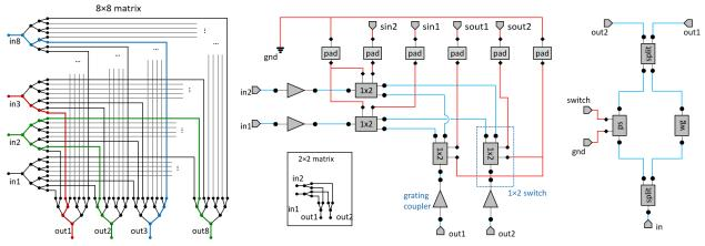
Fig. 2. Left: an  $8 \times 8$  non-blocking crossconnect matrix with multicasting capability. Middle: a reduced  $2 \times 2$  matrix with the corresponding photonic-electronic circuit. Note that the topology of this circuit requires at least one crossing. Right: The subcircuit schematic of the  $1 \times 2$  switch.
