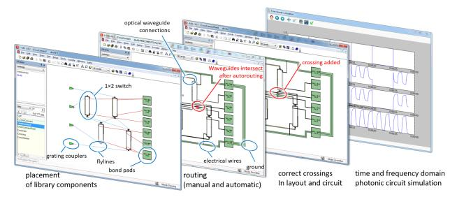
Fig. 3. Constructing the  $2 \times 2$  crossbar switch of Fig. 2. Left to right: placing and logically connecting the library components; generating waveguides and electrical wires; correction of the waveguides by introducing a crossing; Time-domain simulation of the switching behavior.
