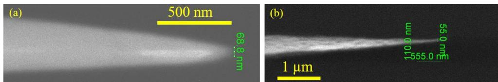
Figure 1. SEM images of fabricated silica nano-tip fiber (a) with organic overlayer, (b) without organic overlayer.
