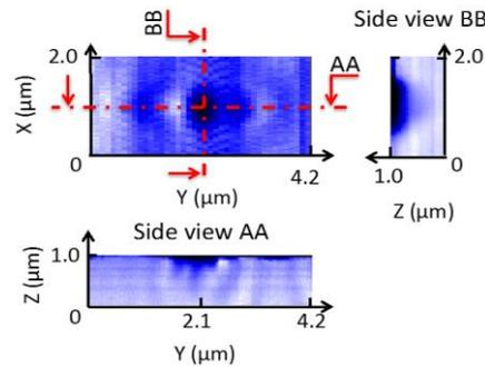
Figure 3. Three-dimensional map of the intensity variation induced by the interaction between the nano-tip fiber and the L3 cavity.
