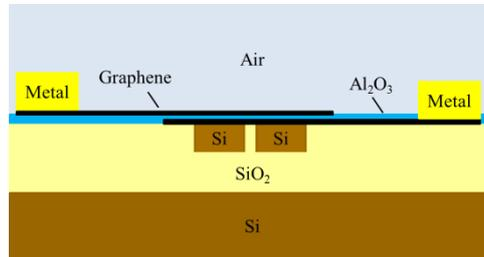
Figure1. A schematic of the double layer graphene-on-Si slot waveguide optical switch.
