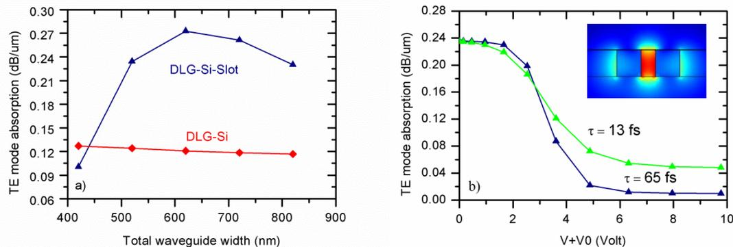
Figure 2. a) The TE mode absorption at the Dirac point versus the total waveguide width ( $2 \times$  Si section width + slot section width), the graphene scattering time is 65 fs b) The TE mode absorption for the
