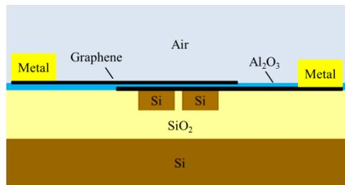
Figure1. A schematic of the double layer graphene-on-Si slot waveguide optical switch.
