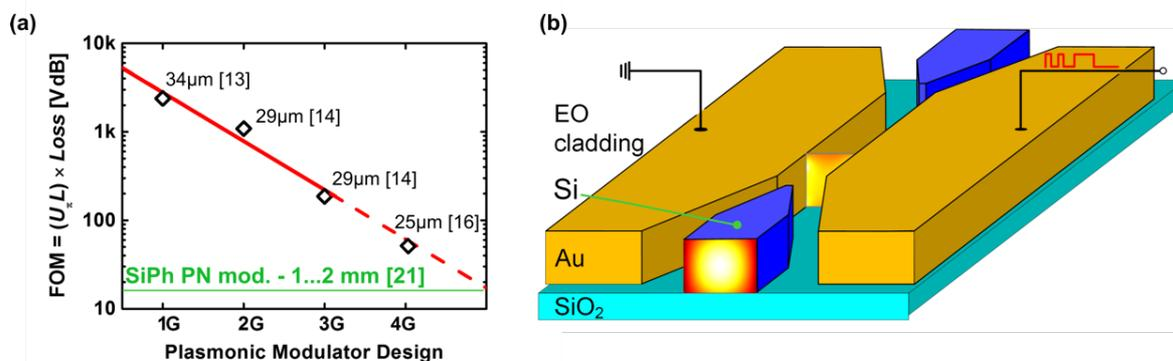
Fig. 1. Plasmonic-organic hybrid technology and an overview of the figure-of-merits (FOM) reported previously. (a) Performance improvement reported for POH modulators over the last several years. In the calculation of the FOMs, only the optical losses in the plasmonic section are only considered. (b) The schematic of the POH phase modulator comprising two metallic taper mode converters and metallic slot waveguide.
