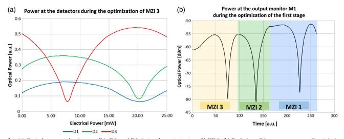
**Fig. 4.** (a) Optical power at the detectors D1, D2, and D3 during the optimization of MZI 3. (b) Evolution of the output power at Out 1 during the optimization of the first stage. The optical power was recorded from the monitor M1, which taps the light from Out 1.
