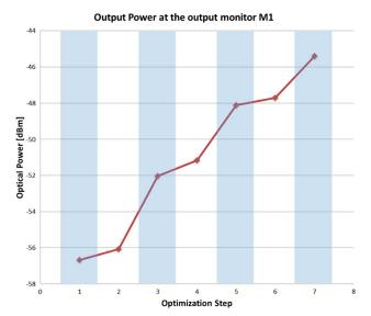
**Fig. 8.** Optical power at monitor M1, placed at Out 1. The blue region represents steps where a common-mode optimization step happened, while the white regions are refer to differential optimization steps.
