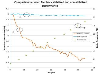
**Fig. 10.** Normalized optical power at the output of the circuit showing the stability of the circuit over time. The optical power was measured over a time span of 60 min while the temperature of the circuit was gradually incremented from 20°C to 30°C. The plot shows that the circuit, when operating using the feedback loops, can maintain stability of operation over a long period of time and with temperature change.
