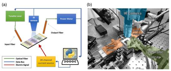
Fig. 3. (a) Schematic diagram of the experimental setup. (b) Picture of the setup.
