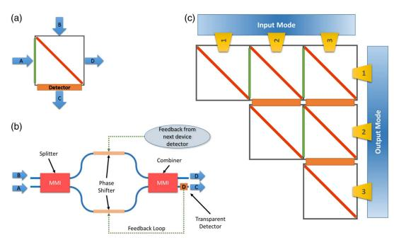
**Fig. 1.** (a) Representation of an individual cell of the circuit with two inputs (A and B) and two outputs (C and D). The green rectangle is a tunable phase shifter and the red rectangle is a semi-transparent mirror with tunable reflectivity. The orange rectangle is a "transparent" photodetector. (b) Mach–Zehnder implementation of the unit cell. (c) A discrete representation of the proposed device from cascaded discrete unit cells.
