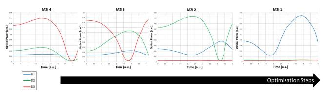
Fig. 7. Power level at the detectors D1, D2, and D3 during the optimization of MZI 4 to MZI 1.
