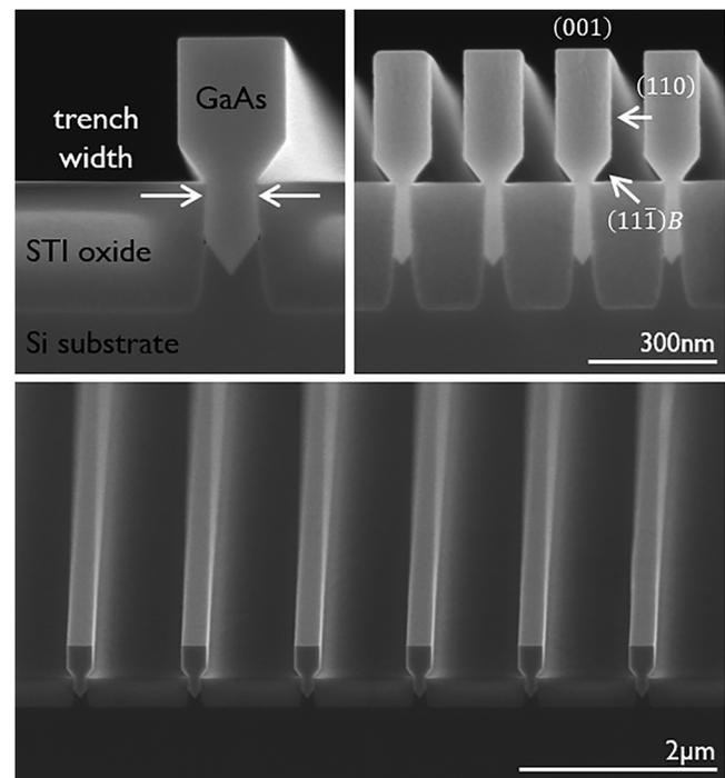
FIG. 1. SEM pictures of box shaped ridges integrated on STI-patterned Si wafers. Top left: Cross-section of a 100 nm wide trench. Top right: Cross-section of 20 nm wide trenches. Bottom: inclined top-view of a 100 nm trench array. The facet nomination is the same for the GaAs growth in narrow and wide trenches.
