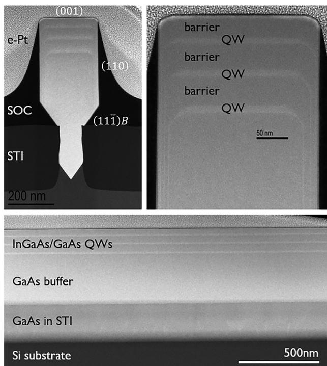
FIG. 2. HAADF-STEM pictures of a box shaped GaAs ridge with three InGaAs QWs. Top left: Cross-section of the full ridge. Top right: Higher magnification of the QW region. Bottom: Transverse section along the trench. The GaAs inside the STI shows a slightly different contrast because some STI oxide was cut out during sample preparation.
