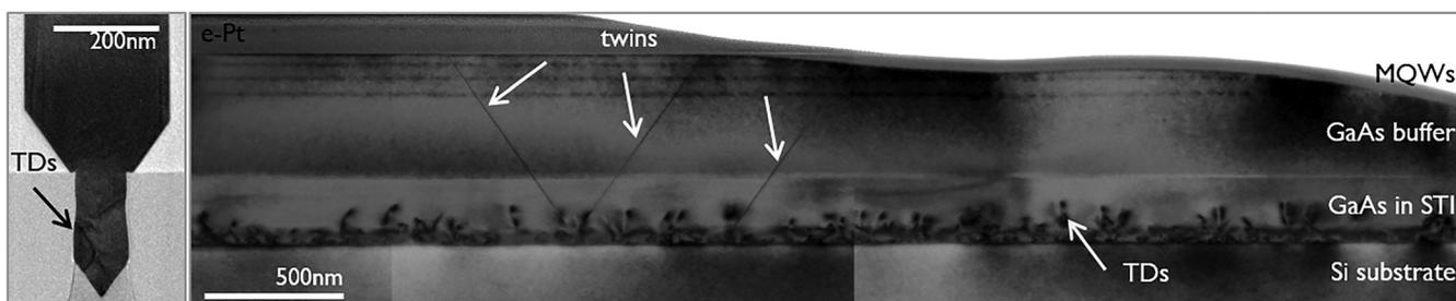
FIG. 3. Left: Cross-section HR-TEM of the GaAs buffer. Right: Combined BF(002) images of a transverse section along the trench. The vertical lines visible in the Si substrate are caused by the image combination. Threading dislocations are clearly visible by the dark blurred contrast, whereas planar defects such as micro twins cause a straight dark line in  $\{111\}$  directions.
