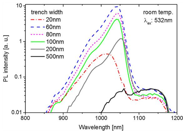
FIG. 4. Room temperature PL spectra from different trench widths in log-scale.
