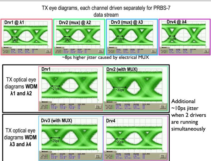
Figure 22.5.4: Measured 20Gb/s TX eye diagrams for each wavelength separately and in 2-WDM configuration.
