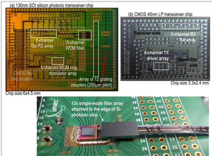
**Figure 22.5.7: Si-photonics and CMOS chip pictures. Flip-chip integrated optical transceiver demonstrator with attached fiber array, glued and wire-bonded to a PCB.**
