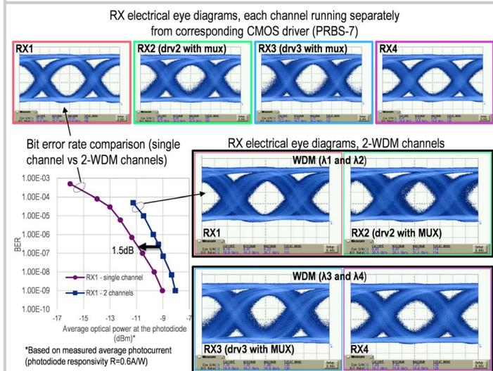
Figure 22.5.5: Measured 20Gb/s RX eye diagrams and BER (single wavelength and 2-WDM operation).
