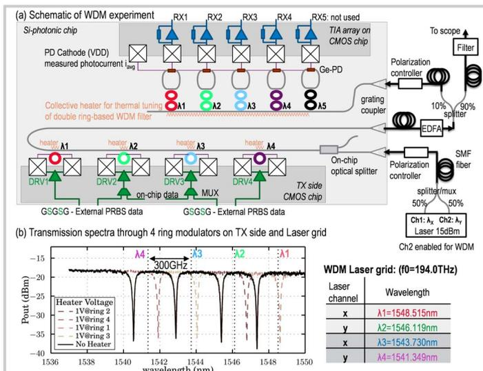
Figure 22.5.1: (a) Schematic of 20Gb/s WDM optical transceiver. (b) Transmission spectra of TX and laser grid settings.
