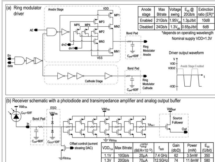
Figure 22.5.3: Schematics and performance tables of the ring modulator driver and TIA for 20Gb/s.
