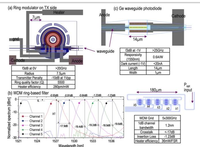
Figure 22.5.2: Key SiPh devices: (a) ring modulator with integrated heater (b) ring-based WDM filter with integrated collective thermal tuning (c) Ge waveguide photodiode.
