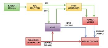
Fig. 3. The measurement setup
