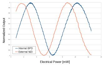
Fig. 4. Comparison between the the output of the on-chip measurement (blue) and the measurement using the external MZI (orange).
