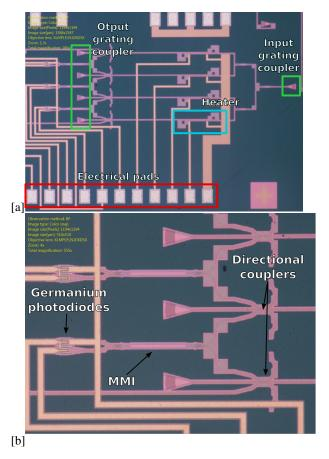
Fig. 2. Microscope image showing (a) the full circuit and (b) a zoom into the directional couplers, the MMI and the germanium photodiodes.
