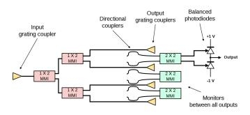
Fig. 1. PLACEHOLDER - Schematic diagram of the circuit.
