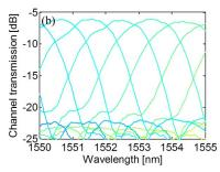
Fig. 2. Measured spectral response of the device. (a) Full spectral order. (b) Detail of the spectral response around the center wavelength. Large intentional cross-talk between the channels is achieved.
