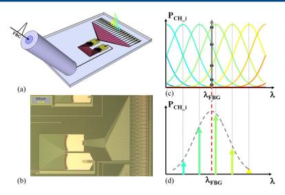
Fig. 1. Operating principle of the interrogator. (a) Sketch of the device. (b) Optical microscope image of the fabricated device. The total footprint is  $2.2\times1.5$  mm. (c) The FBG peak produces a measurable output over several channels. (d) The center of mass of the FBG peak can estimated using the recorded power values if the AWG channel positions are known.
