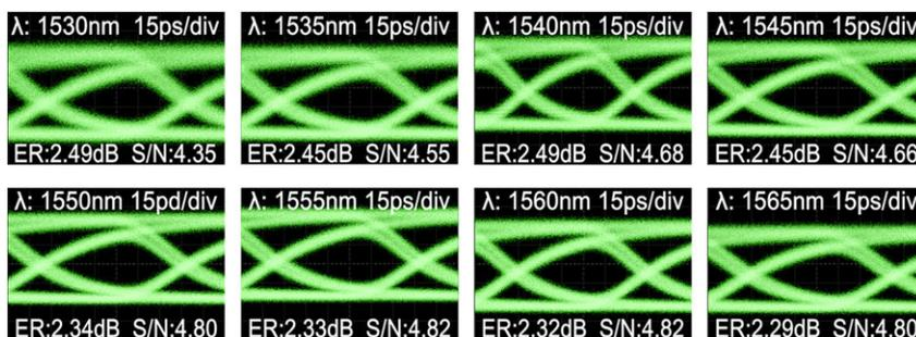
**Figure 12** Optical eye diagrams measured at 10 Gb/s modulation speed for the 50  $\mu\text{m}$  graphene EAM device for wavelengths in the range 1530–1565 nm, using a drive voltage of 2.5  $V_{pp}$  swing and 1.75 V forward bias delivered with a 50  $\Omega$  terminated probe. A dynamic extinction ratio of 2.3 dB or better is obtained for all wavelengths.
