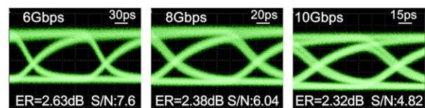
**Figure 11** Optical eye diagrams measured at 1560 nm for the 50  $\mu\text{m}$  graphene EAM device at 6 Gb/s, 8 Gb/s and 10 Gb/s modulation speed, using a drive voltage of 2.5  $V_{pp}$  swing and 1.75 V forward bias delivered with a 50  $\Omega$  terminated probe.
