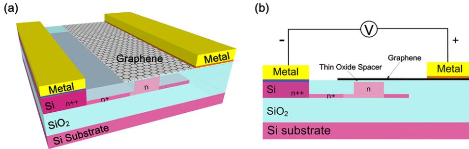
**Figure 1** (a) A 3 dimensional schematic drawing of a single layer graphene electro-absorption modulator (EAM) integrated on SOI platform. (b) Cross section of the graphene EAM.
