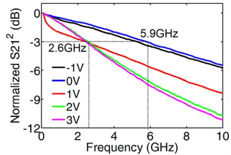
**Figure 10** Measured and normalized electro-optical  $S21$  responses of the 50  $\mu\text{m}$  graphene EAM at different bias voltages showing electro-optical bandwidth of 5.9 GHz in reverse bias and 2.6 GHz in forward bias.
