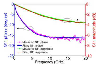
**Figure 9** Measured RF  $S_{11}$  response of the 50  $\mu\text{m}$  graphene EAM at 0 V bias and the fitted curves using an equivalent electrical circuit model.
