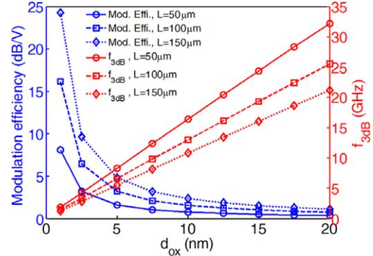
**Figure 5** Calculated modulation efficiencies and electrical 3-dB bandwidths as functions of the thickness of the oxide spacer for different device length of 50, 100 and 150  $\mu\text{m}$ .
