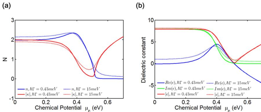
**Figure 2** (a) Calculated complex dielectric constant (real part, imaginary part and magnitude) of graphene as a function of chemical potential at fixed wavelength of 1550 nm for  $\hbar\Gamma = 0.43$  meV and 15 meV. (b) Calculated complex refractive index (real part, imaginary part) of graphene as a function of chemical potential at fixed wavelength of 1550 nm for  $\hbar\Gamma = 0.43$  meV and 15 meV.
