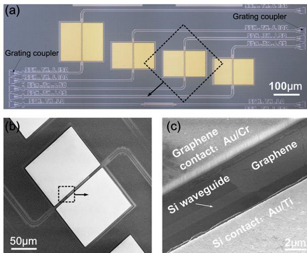
**Figure 6** (a) Optical microscope image of the fabricated graphene EAMs with TM grating couplers for fiber-to-chip optical coupling. (b) Top-view and (c) tilted-view SEM images of fabricated devices.
