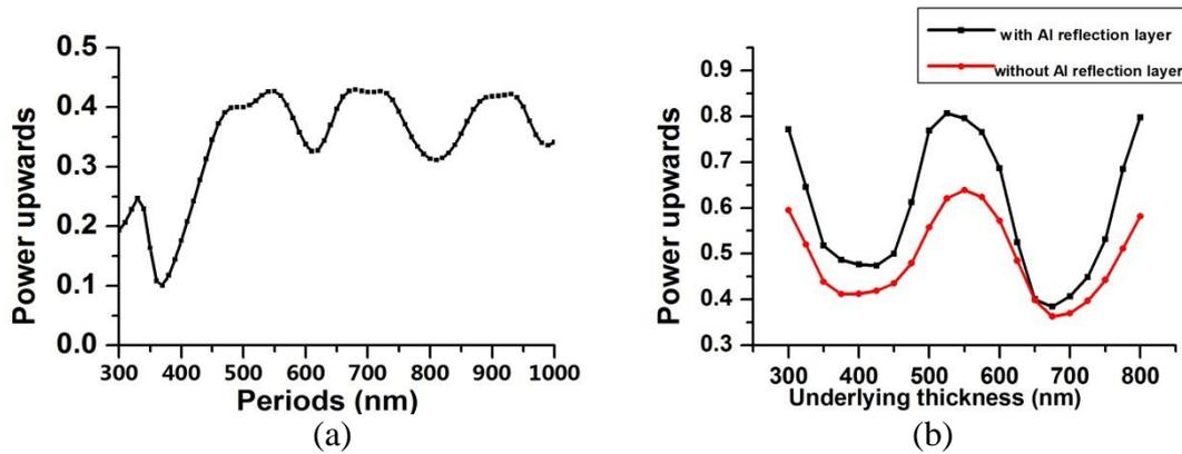
Fig. 2. (a) 2D FDTD simulation results of grating period length vs power upwards. (b) 2D FDTD simulation results of underlying thickness sweep: black one is silicon substrate with Al as reflection layer, red one is silicon substrate without Al as reflection layer
