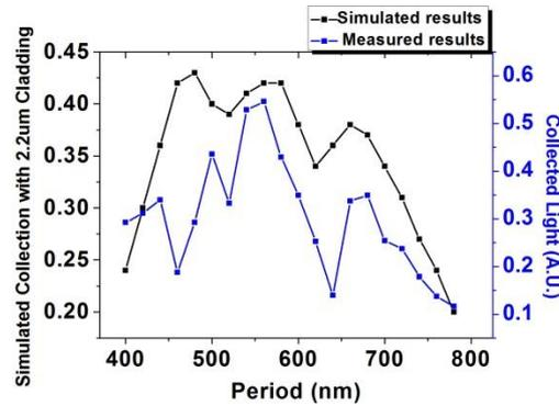
Fig. 8. Measurement results: the black curve is the simulated power couple to a microscopy system with NA=0.65, the underlying thickness is 2.2um as fabricated sample; the blue curve is the measurement results.
