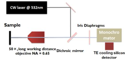
Fig. 7. Schematics of the measurement setup
