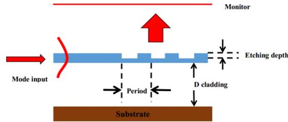
Fig. 1. The schematic of the grating coupler
