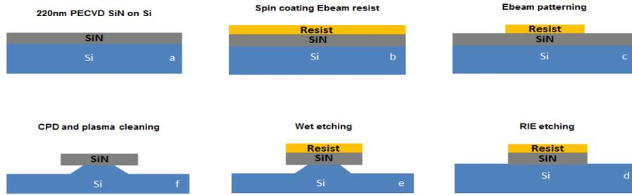
Fig. 5. Schematics of the fabrication flow of ultra-compact grating coupler
