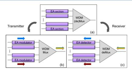
Fig. 1. (a) Present six-channel WDM optical transceiver architecture, which can be used as (b) transmitter or (c) receiver.
