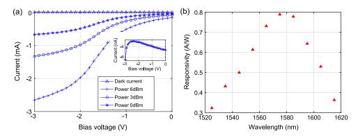
Fig. 6. (a) Static response of one EA detector section. Different curves are for different input light powers in the silicon waveguide. (Inset) Zoom-in view of the dark current. The operation wavelength is 1563.9 nm. (b) Responsivity of the EA detector section as a function of wavelength. The bias is -3 V.
