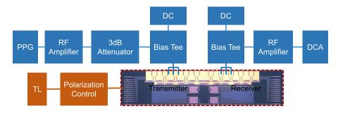
Fig. 10. Measurement setup for the on-chip interconnect characterization.
