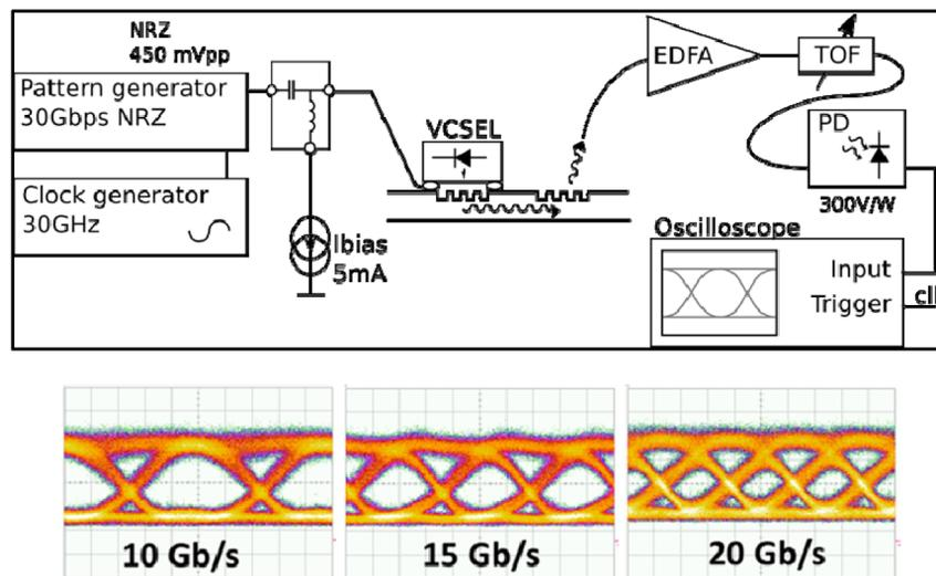
Fig. 5. Illustration of the experimental set-up used for performing NRZ transmission measurements on flip-chip bonded assemblies (top) and eye diagrams recorded for the bonded VCSELs at 10, 15 and 20 Gb/s (bottom).
