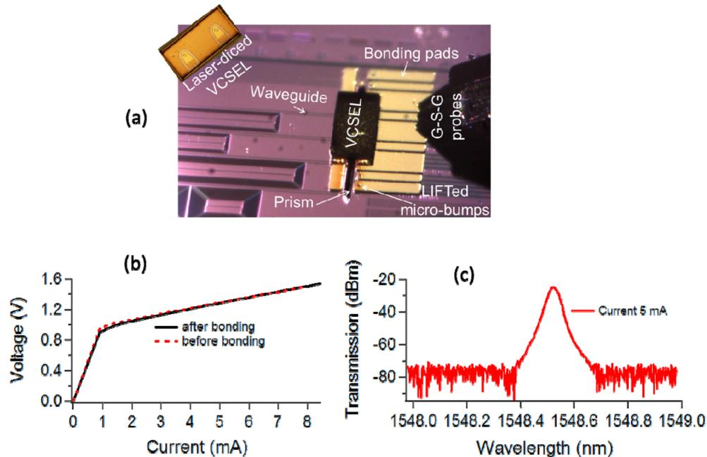
Fig. 3. (a) Optical microscope image of the final VCSEL-to-SOI chip bonded assembly, with inset showing a 1 x 2 laser-diced VCSEL chip; (b) I-V characterization curves for the VCSEL prior and post bonding and (c) Optical spectrum of the bonded VCSEL measured through the output GC of the waveguide.
