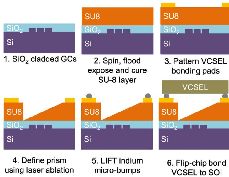
Fig. 1. Schematic for the process flow describing SU8 prism fabrication and VCSEL flip-chip integration on SOI GCs.
