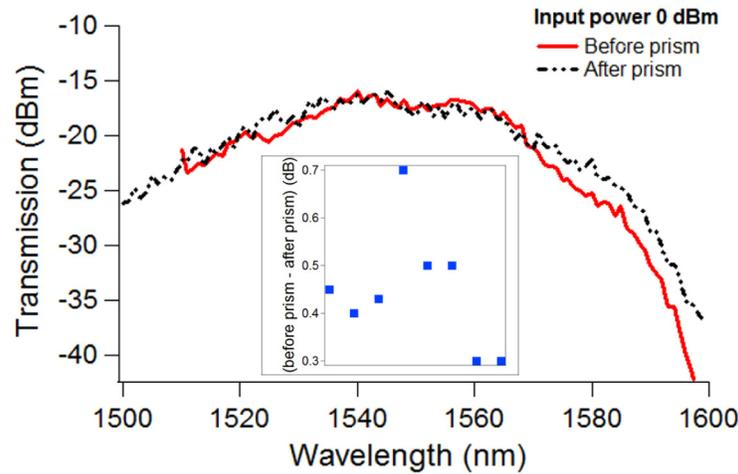
Fig. 4. Comparison between the transmission curves recorded before and after SU8 prism fabrication on top of SOI GCs. The inset shows a plot, indicating the statistical distribution of the prisms' performances at 1550 nm over 8 different samples.
