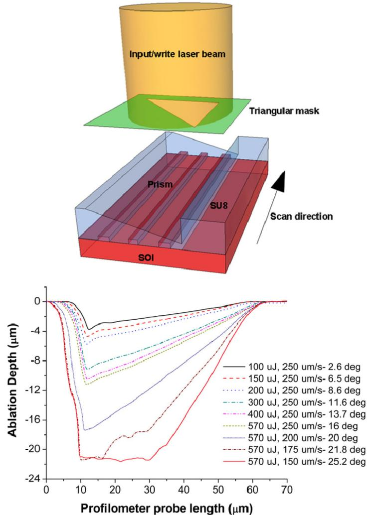
Fig. 2. (top) Schematic of non-uniform laser ablation technique for SU8 prism fabrication on top of GCs, and (bottom) Variation of SU8 ablation depth (prism angle) w.r.t laser energy/writing speed as measured by a profilometer.
