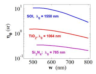
Fig. 9. The conversion efficiency  $\eta_0$  of slot waveguides with s = 100 nm as a function of total waveguide width w for different material systems and corresponding excitation wavelengths. Note that y-axis in log scale.
