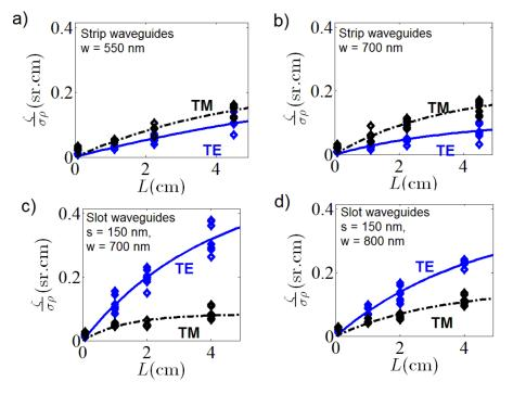
Fig. 3. Experimental data from the Raman peak of IPA at 819 cm<sup>-1</sup> a) strip waveguides, w = 550 nm, b) strip waveguides, w = 700 nm, c) slot waveguides, w = 700 nm, s = 150 nm d) slot waveguides, w = 800 nm, s = 150 nm. Diamonds: experimental values. Lines: LSE fit of  $\zeta$  (L) as per Eq. (1). Black diamond and black dashed lines: TM polarized excitation and collection. Blue diamond and blue solid lines: TE polarized excitation and collection.
