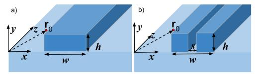
Fig. 1. Schematic of a dielectric a) strip and b) slot waveguides defined by a core of higher refractive index (Si<sub>3</sub>N<sub>4</sub>, TiO<sub>2</sub> or silicon) patterned on a lower index bottom cladding (typically silicon dioxide). The scattering particles are assumed to be embedded with a uniform density in the upper cladding (colorless region). A particle at position  $\mathbf{r}_0$  is shown for both cases for theoretical analysis in the Appendix.
