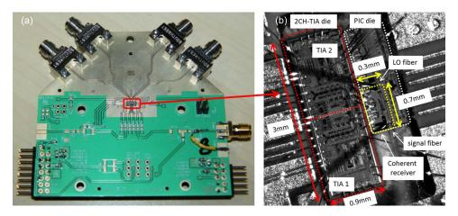
Fig. 8. (a) View of the PCB used for testing purposes with the integrated silicon photonic coherent receiver and TIA array. (b) Close-up of the wire bonded electronic and photonic die (comprising the 0.3 mm by 0.7 mm coherent receiver) on the PCB.
