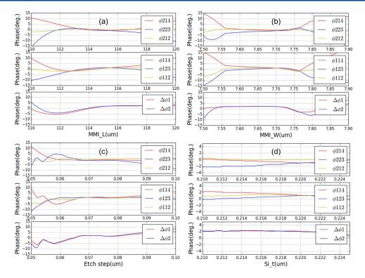
Fig. 3. Tolerance analysis on the phase relations of the ultra-compact 90° hybrid used in this work. (a) Influence of the length of the MMI coupler; (b) influence of the MMI width; (c) influence of the MMI etch depth; (d) influence of the silicon waveguide thickness (1550 nm wavelength, TE polarization).
