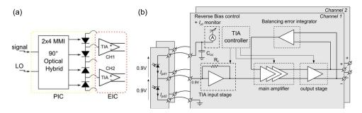
Fig. 6. (a) Block diagram of the integration of the silicon PIC with the 2-channel TIA array. (b) TIA architecture and on-chip biasing scheme and decoupling of photodiodes.
