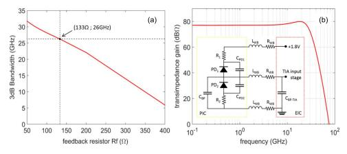
Fig. 7. (a) Simulation of the TIA bandwidth as a function of the trans-impedance with indication of the used transimpedance setting (133  $\Omega$ ) and resulting 3 dB-bandwidth (26 GHz). (b) Simulated trans-impedance gain of the TIA as a function of frequency for a trans-impedance of 133  $\Omega$ , as is used in the experiment. The equivalent circuit of the balanced photodiodes taking into account the parasitic capacitance of the pads and the inductance of the bond wire is shown in the inset.
