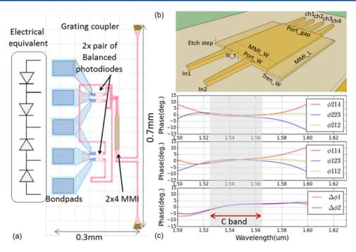
Fig. 2. (a) Layout of the single polarization coherent receiver with a footprint of 0.3 mm by 0.7 mm. (b) Layout of the 90° hybrid defined on imec's iSIPP25G platform. (c) Simulation of the wavelength dependence of the 90° hybrid.
