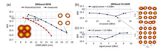
Fig. 10. (a) BER versus OSNR curve for 28 Gbaud QPSK. (b) 28 Gbaud 16-QAM BER versus LO power together with representative constellation diagrams illustrating the BER degradation at higher LO power. (c) 28 Gbaud 16-QAM BER versus signal power. Below FEC operation is obtained.
