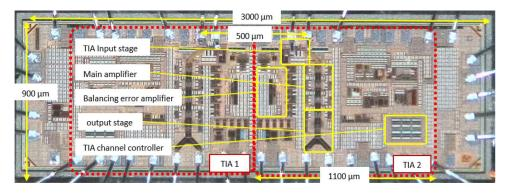
Fig. 5. Top-view of the two-channel TIA with an indication of the position of the different functional blocks.
