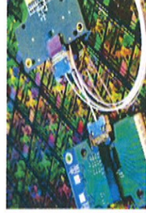
Drastic reduction of energy consumption through optical fiber interconnect and silicon photonic chips
