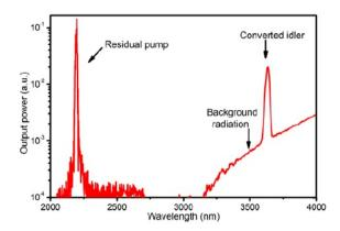
**Fig. 19.** The output spectrum of the wavelength translator when it is seeded with a CW probe at 1565 nm. A strong signal at 3635 nm can be seen above the thermal background of the detector. Adapted from reference [65].
