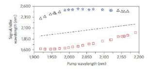
**Fig. 15.** The phase-matched signal (squares) and idler (stars and triangles) wavelengths as a function of the pump wavelength in the four wave mixing process in the silicon waveguide. The stars represent the calculated idler location (from the measured signal wavelength) as they are outside the bandwidth of the OSA. Adapted from reference [63].
