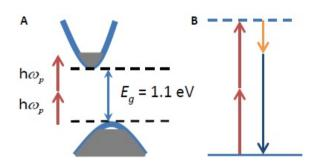
**Fig. 1.** (a) The two-photon absorption process: the combined energy of two photons generates a free carrier. (b) The degenerate fourwave mixing process in which a lower energy idler and high energy signal photon are created by the annihilation of two pump photons.
