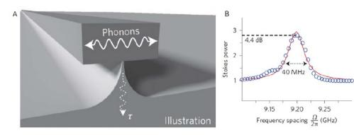
Fig. 26. Phonon-photon coupling in a silicon photonic waveguide. (a) Illustration of the partially underetched waveguide. (b) The on/off gain of a detuned signal by a 35 mW pump.
