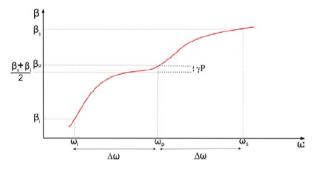
**Fig. 7.** Phase-matching for a very large signal and idler detuning. When  $\beta_{4p} < 0$  and  $\beta_{2p} > 0$ , there is only one pair of signal and idler frequencies that are phase-matched with the pump frequency.
