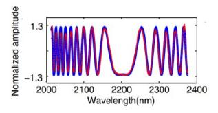
**Fig. 4.** The fringes recorded by the optical spectrum analyzer after the interferometer (red: recorded fringes; blue: fitted theoretical fringe pattern). The fringes allow to extract the dispersion profile of the waveguide. Adapted from reference [19].
