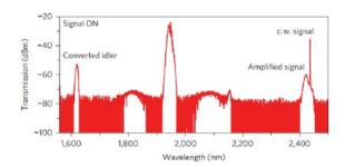
**Fig. 16.** The output spectrum after the signals (1946 nm pump pulses and a 2440 nm CW signal) have propagated through the silicon waveguide. In this case, the mid-infrared CW signal is converted to the telecom wavelength band. Adapted from reference [63].
