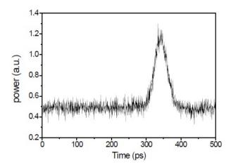
**Fig. 20.** Amplification of a telecom probe. A temporal trace recorded by a fast photo-detector in the telecom band. The instantaneous amplification after propagating through the silicon waveguide visible (shown in the inset of Figure 18) of the telecom probe signal is clearly visible.
