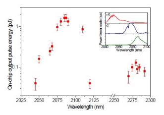
Fig. 25. The output power of our OPO, as shown in the inset of Fig. 24 at different idler wavelengths. Adapted from reference [68].
