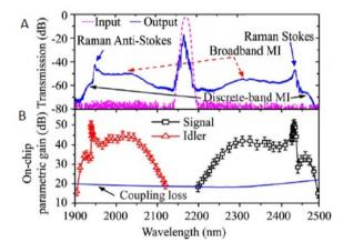
**Fig. 13.** Parametric ampification in the mid-infrared using the waveguide described in Fig. 12, pumped using ps pulses centered around 2120 nm. (a) The spectrum of the pump pulses before and after passing through a 2 cm long waveguide; (b) amplification and conversion efficiency as a function of seed wavelength. The total insertion loss of the chip is shown in blue. Adapted from reference [58].
