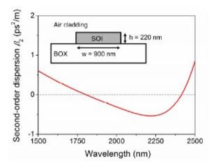
**Fig. 12.** The group velocity dispersion of the waveguide used for the mid-infrared parametric amplifier experiment as well as for the OPO experiment discussed in Section 3.3. The inset shows a cross-section of the waveguide. Adapted from reference [57].
