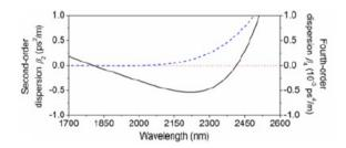
**Fig. 14.** The simulated second (black line) and fourth order (blue dashed line) dispersion of the 900 nm wide silicon waveguide. The sign of the second and fourth order dispersion are opposite in a band between 1810 and 2410 nm. Adapted from reference [63].
