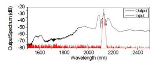
**Fig. 21.** Supercontinuum generation in a 900 nm wide and 220 nm thick silicon waveguide. The input and output spectrum of the pulse train shows the dramatic spectral broadening of the pulses after propagating through a 2 cm long nanowire waveguide. Adapted from reference [57].
