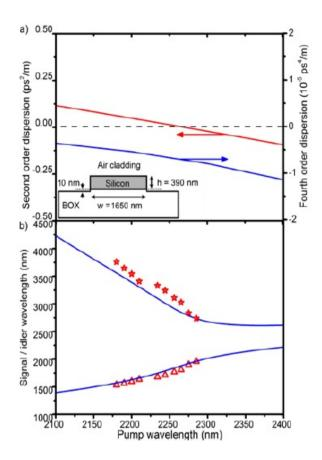
**Fig. 18.** (a) The simulated second and fourth order dispersion of the silicon waveguide shown in the inset. (b) The phase-matched signal (triangles) and idler (stars) wavelengths as a function of the pump wavelength for this waveguide. The blue line is the theoretical prediction of phase-matched idler and signal pairs as a function of pump wavelength. Adapted from reference [65].
