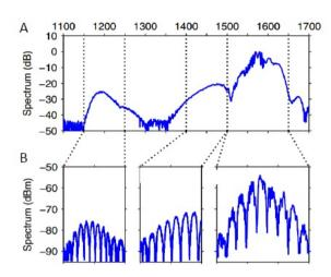
**Fig. 9.** Coherent supercontinuum generation in a silicon waveguide using fs pulses . a) The spectrum a) and b) the fringes obtained with the interferometric setup of Figure 10 show that the supercontinuum is coherent. Adapted from reference [26].
