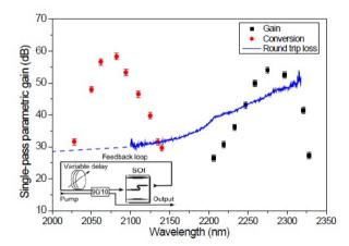
**Fig. 24.** The parametric gain of the photonic wire waveguide and the round trip-losses of the cavity. The gain can overcome the losses over a broad wavelength band. The inset shows a schematic of the experimental setup. The cross-section of the waveguide is the same as shown in the inset of Figure 12. Adapted from reference [68].
