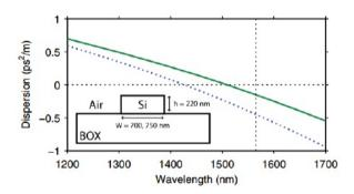
**Fig. 8.** The group velocity dispersion of the fundamental TE mode of a silicon waveguide as a function of wavelength for a 700 nm wide waveguide (dotted line) and a 750 nm wide waveguide (solid line). The inset shows the waveguide cross-section. Adapted from reference [26].
