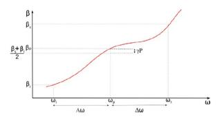
**Fig. 6.** Phase-matching for a large signal and idler detuning. When  $\beta_{4p} > 0$  and  $\beta_{2p} < 0$  there is, in addition to the solution in the vicinity of the pump frequency,  $\omega_p$ , a second pair of signal and idler frequencies which are phase-matched with the pump frequency.
