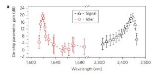
**Fig. 17.** Amplification and conversion efficiency of the silicon wavelength translator (see Figs. 15 and 16) as a function of the midinfrared signal wavelength. Adapted from reference [63].
