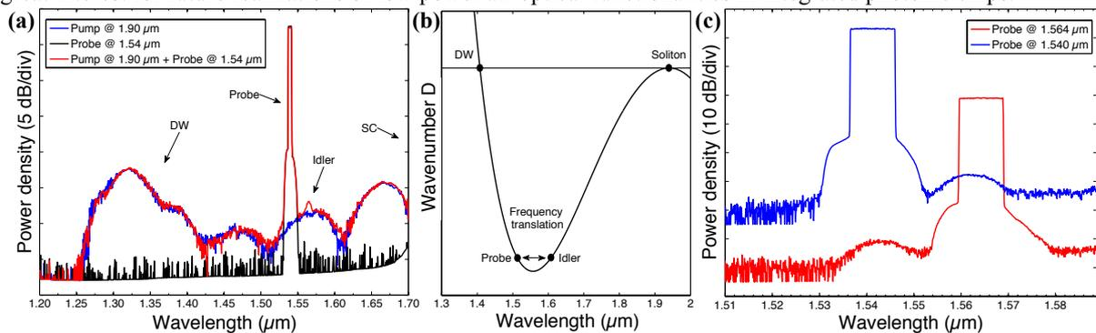
**Fig. 1** (a) Experimental output spectra for the demonstration of the optical analog of an event horizon. (b) Wavenumber  $D$  as a function of the wavelength computed from the theoretical dispersion curve. (c) Experimental spectra highlighting the interchangeability of probe and idler. Note that the blue spectrum has been shifted by 20 dB for clarity.
