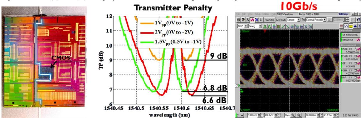
Figure 4. Left: Flip-chip 40nm CMOS driver circuit on top of a silicon photonics transmitter circuit with microring modulators. Middle: Transmitter penalty as function of wavelength for various voltage swing. Right: 10dB extinction ratio at 10Gb/s modulation realized with a 40nm driver operating at  $V_{DD}=1.1\text{V}$ .
