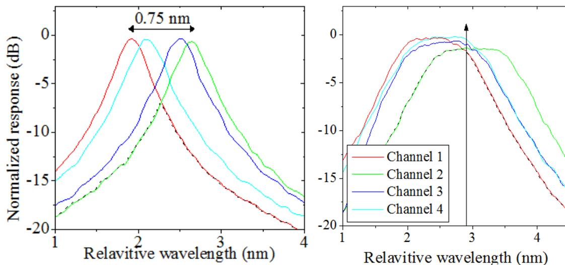
Figure 6. A four channel demultiplexer spectral response for (left) single ring and (right) double ring filters. The responses wavelength is normalized to the designed channel center wavelength.
