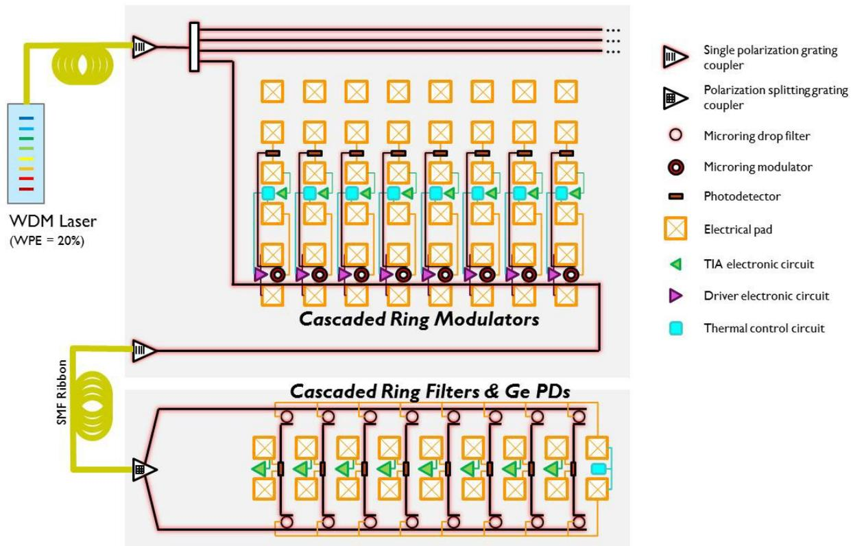
Figure 1. Schematic of a WDM architecture schematic based on micro-ring resonators and grating couplers.
