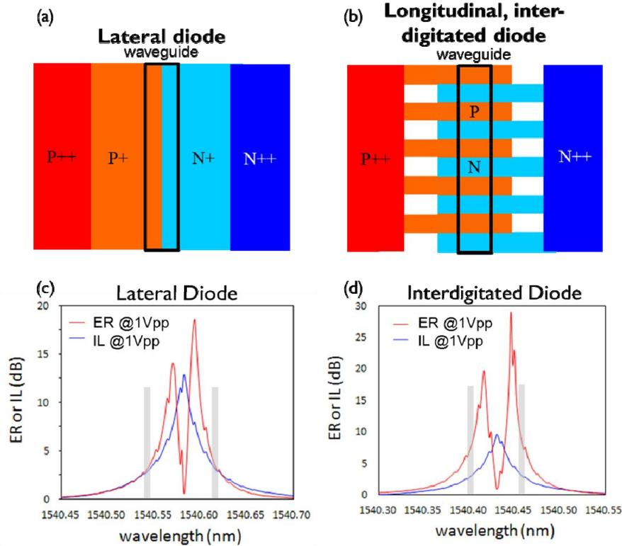
Figure 3. Top-down waveguide schematic of (a) a lateral p-n diode and (b) a interdigitated diode. The extinction ratio and insertion loss for a  $1.0\text{V}$  peak-to-peak are shown for lateral (c) and longitudinal (d) diode configuration. In (c) and (d) the grey band illustrates the operating range with minimum transmitter penalty.
