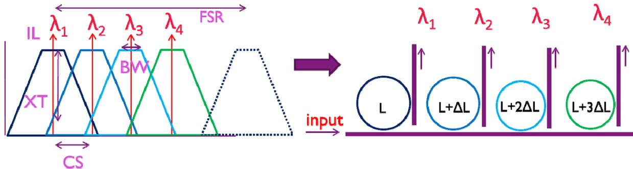
Figure 5. Demultiplexer spectrum design and implementation in microring resonators.
