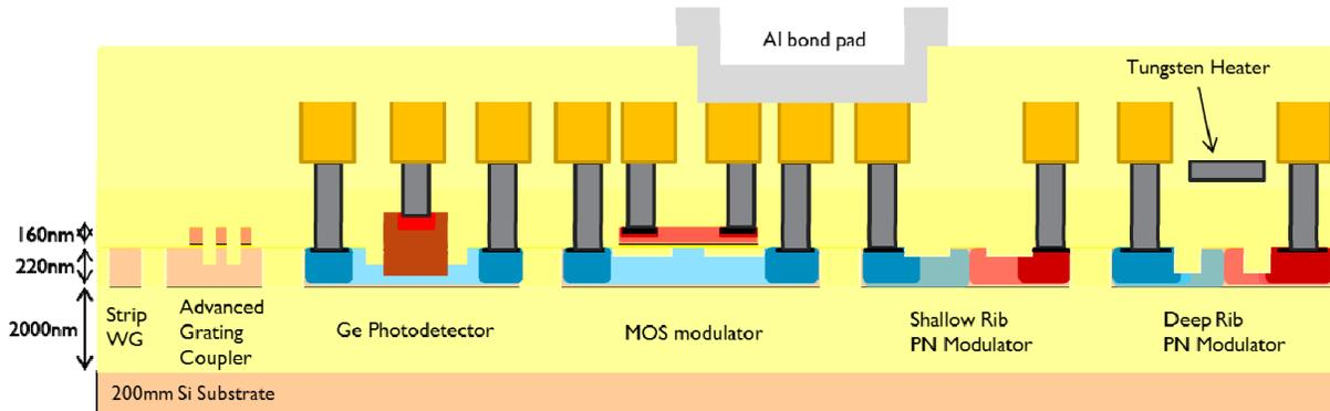
Figure 2. Cross section schematic of the silicon photonics integrated platform combining high quality passives, silicon modulators, integrated heaters and Ge-on-Si photo-detectors.
