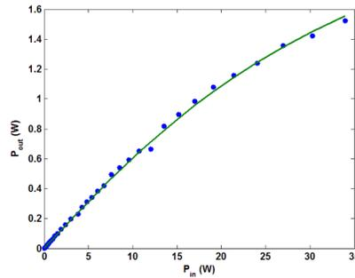
Fig. 3. The measured output peak power as a function of the input peak power (circles) and the best-fit using Eq. (2) which gives a  $\alpha_3$  value of  $2.5 \times 10^{-2} \text{ cm}^3 / \text{GW}^2$ .
