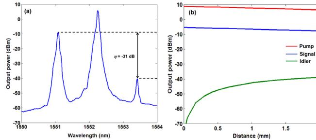
Fig. 5. (a) The measured output spectrum of the pump, signal and idler showing a conversion efficiency of  $-31 \text{ dB}$  and (b) the simulated evolution of the pump, signal and idler power (taking into account  $-7.5 \text{ dB}$  outcoupling efficiency) along the waveguide for  $\gamma = 475 \text{ W}^{-1}\text{m}^{-1}$ .
