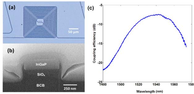
Fig. 1. (a) A 1 cm long InGaP waveguide with small footprint due to the high index contrast; (b) the SEM cross-section of the InGaP waveguide with measured dimensions of 630 nm x 250 nm; (c) the coupling efficiency of the shallow etched grating as a function of wavelength showing a maximum efficiency of  $-7.5$  dB at 1540 nm (TE polarization).
