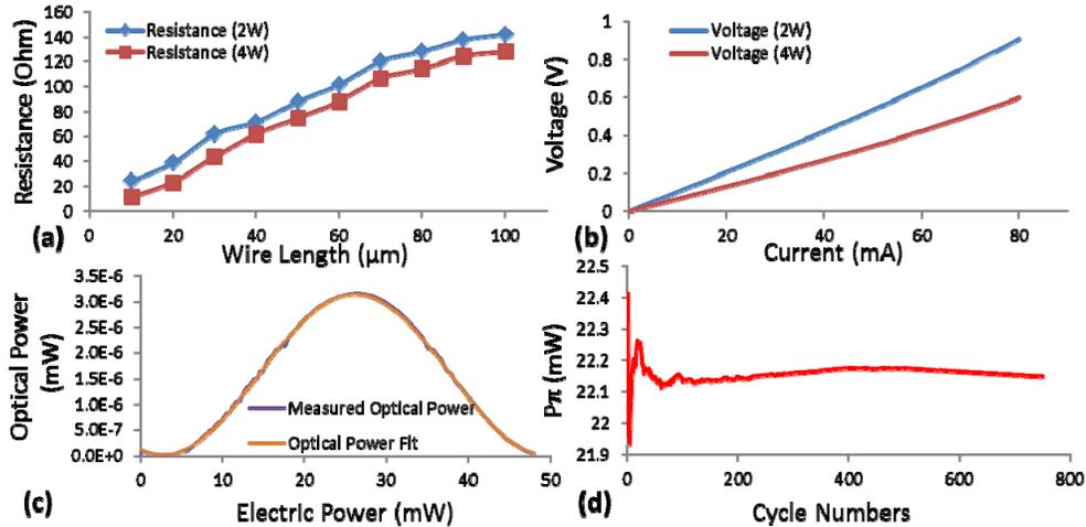
Fig. 3. (a) Length versus resistance plot for  $0.6\mu\text{m}$  wide heater wire. (b) IV characteristics of a heater during operation. (c) Output optical power of MZI versus applied electrical power. (d) Variation of power efficiency over multiple cycles.
