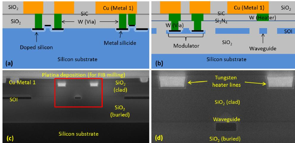
Fig. 1. Cross sections of (a) Typical CMOS stack with front-end and back-end. (b) SOI-photonics stack with modulator and W heater. (c) SEM image of SOI-photonics device cross section. (d) W heaters and waveguide.
