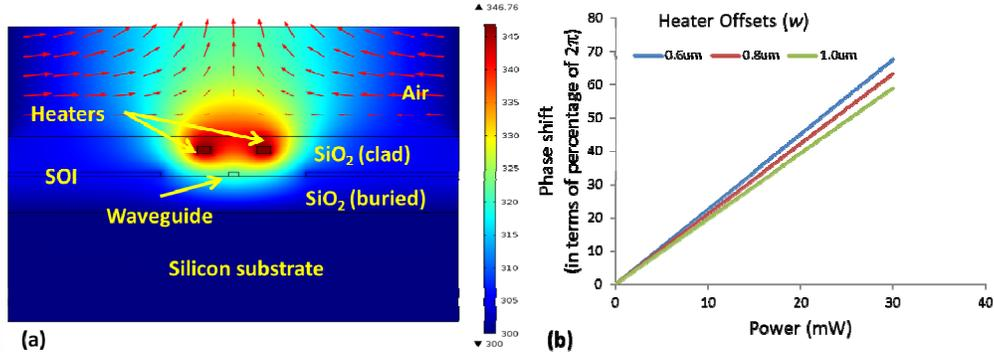
Fig. 2. (a) Simulated temperature profile of device cross section model. (b) Simulated phase shift versus applied electrical power for different heater offsets ‘w’, defined as the horizontal distance between inward edges of heater line and the waveguide.
