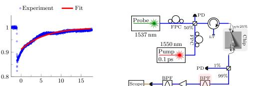
FIG. S1. Measurement of the free-carrier lifetime. a, Oscilloscope trace of the probe power. The pump pulse arrives at t = -1 ns. We start the fit a nanosecond later to avoid fitting to photodiode ringing artifacts. b, Pump-probe set-up used to obtain the trace. The band-pass filter (BPF) has more than 50 dB extinction at 1550 nm.
