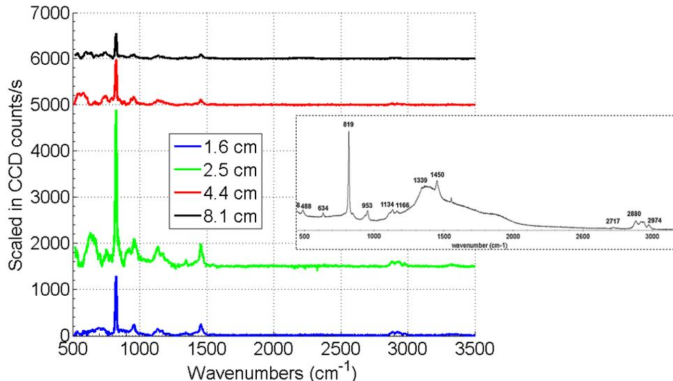
**Figure 1** The background subtracted Raman spectra of IPA measured using photonic waveguides of lengths 1.6, 2.5, 4.4 and 8.1 cm (from bottom to top respectively, shifted vertically for clarity with zero at 3200  $\text{cm}^{-1}$ ). Raman spectrum of IPA [4] is provided in the inset for comparison.
