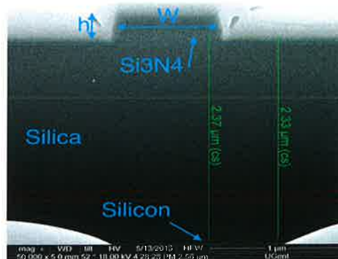
Figure 1: Cross section view of \text{Si}_3\text{N}_4 waveguide discussed in this article. Typically we use h=220 nm and w= 700 nm.
