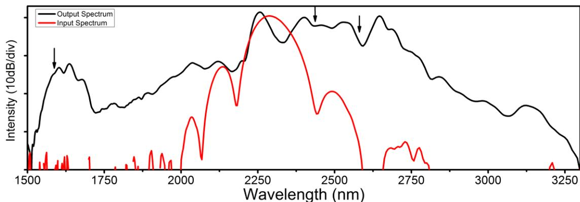
Figure 2: The input and output spectrum of the short pulses travelling through the 1 cm long silicon waveguide. The arrows indicate at which wavelength the coherence is measured.
