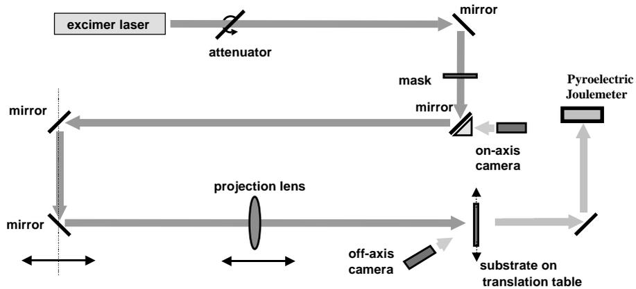
FIG. 2. Laser ablation set-up.
