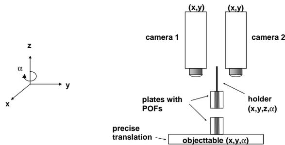
FIG. 6. The 'virtual alignment' set-up.
