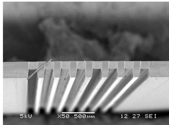
FIG. 3. Array fabricated with moving aperture method in PC at 248 nm (left), array with hybrid mask method in PMMA at 193 nm.
