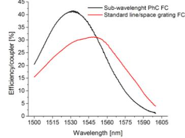
Fig. 3 Sub-wavelength fiber-chip coupler efficiency in comparison with standard line/space grating.
