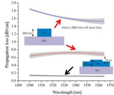
Fig. 2 Propagation loss of a 457 nm wide photonic wire (red curve) and a 700 nm wide ridge waveguide (black curve) in comparison with imec's 200 mm reference wire loss (black curve). The measurement error is indicated by means of grey band.
