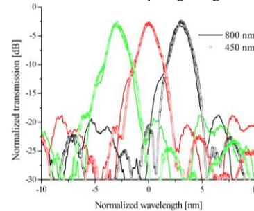
Fig. 4 Normalized transmission spectrum of 3 adjacent channels from 8X400 GHz AWGs with (—) 450 nm an (o) 800 nm delay arm wire width.
