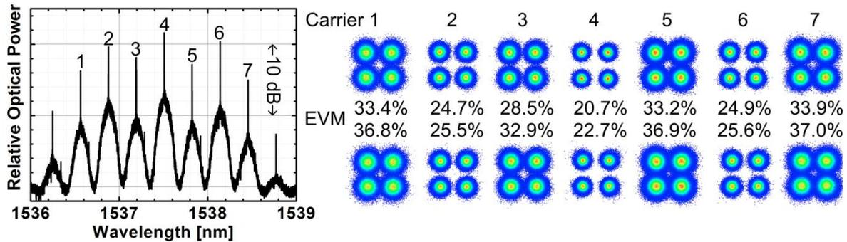
**Fig. 3:** Data transmission results: Data transmission of 784 Gbit/s using QPSK signals on 7 carriers generated by an integrated SOH comb source. Comb spectrum (left) and constellation diagrams for all channels and both polarization are depicted along with measured EVM values. BER below hard-decision threshold are achieved for all signals.
