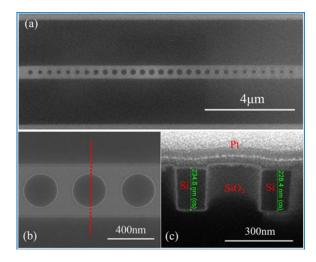
Fig. 4. SEM images of fabricated SOI nanocavity: (a) top view of the whole cavity, (b) enlarged view of holes, and (c) FIB cross-sectional image of a circular hole.
