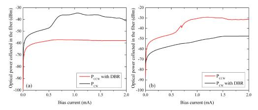
Fig. 8. LI characteristics of microdisk lasers A and B with a diameter of 7.5μm. The plotted optical power is collected in optical fibers on both sides of the WGs. (a) Microdisk laser A coupled to a WG where the DBR has a period of 300nm. (b) Microdisk laser B coupled to a WG where the DBR has a period of 290nm.
