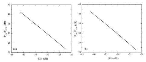
Fig. 7. Ratio of optical powers in the CW and the CCW modes as a function of the ratio of linear coupling between the modes over the amount of external reflection from the bus waveguide induced by the DBR. (a) For a phase  $\Phi = 2\pi$  and values of r between 0.01 and 1.
