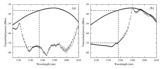
Fig. 10. Transmission characteristics of a WG where the DBR has a period of 300nm (a), and of a WG where the DBR has a period of 290nm (b). The transmission characteristic of a straight WG of the same sample, acting as reference, is systematically plotted.
