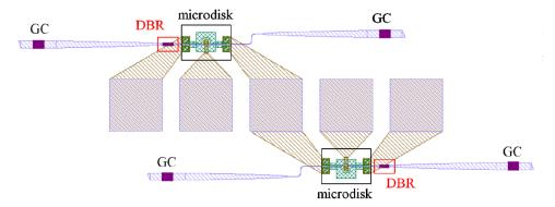
Fig. 2. Design of the fabricated microdisk lasers. The DBR structure on the top WG has a period of 300nm, while the one on the bottom WG has a period of 290nm.
