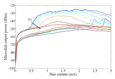
Fig. 11. LI curves of laser B under continuous wave operation at elevated temperatures. The slope efficiency decreases and the threshold current increases at higher temperatures. The power is the fiber coupled output power.
