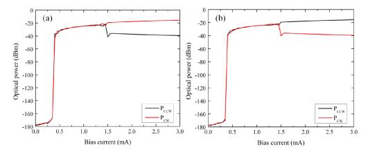
Fig. 4. Bifurcation diagrams of a 7.5μm diameter disk. The optical power in the CW mode is plotted in red, and the optical power in the CCW mode is plotted in black. Depending on initial conditions, one of the modes becomes dominant and suppresses the other at high bias current ((a) The CW mode becomes dominant, (b) The CCW mode becomes dominant).
