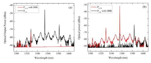
Fig. 9. Spectra of microdisk lasers A and B with a diameter of  $7.5\mu m$ . The plotted optical power is collected in optical fibers on both sides of the WGs. (a) Microdisk laser A coupled to a WG where the DBR has a period of 300nm. (b) Microdisk laser B coupled to a WG where the DBR has a period of 290nm.
