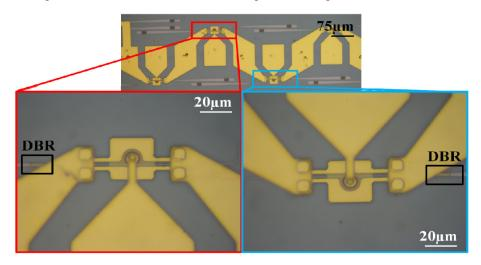
Fig. 3. Microscope pictures of the fabricated devices. The DBR structure can be seen on one side of the waveguide.
