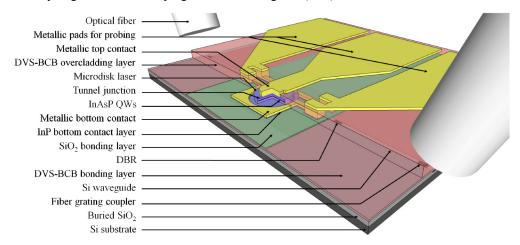
Fig. 1. Schematic view of an InP-based microdisk laser heterogeneously integrated on SOI. The laser emission under electrical pumping of the microdisk evanescently couples to an underlying Si WG. The light is coupled out of the chip using grating couplers, and is collected with optical fibers. A DBR structure can be found on one side of the WG.
