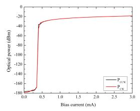
Fig. 5. Bifurcation diagrams of a 7.5µm diameter disk: no gain suppression has been taken into account in the simulation. The optical power in the CW mode is plotted in red, and the optical power in the CCW mode is plotted in black. Unidirectional operation of the laser is not achieved without gain suppression in the microdisk cavity.
