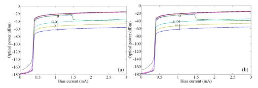
Fig. 6. Bifurcation diagrams of a 7.5 $\mu$ m diameter disk coupled to a straight waveguide where a Bragg reflector is implemented on the CCW propagation direction of the system. All the power is coupled to the CW mode as soon as an external reflection is added to the system. (a) Bifurcation diagrams with a phase  $\Phi = 2\pi$  for increasing values of r. (b) Bifurcation
