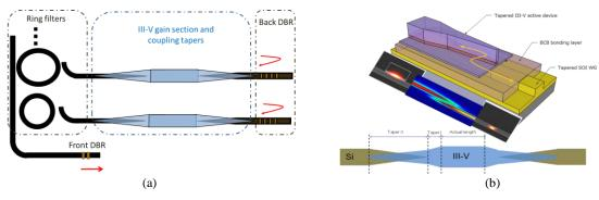
Figure 1: (a) Device layout of the realized III-V/silicon multi-wavelength laser; (b) sketch of the adiabatic spot-size converter used for optical coupling between the III-V amplifier waveguide and silicon waveguide layer.
