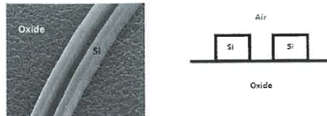
Figure 1: Top view (left) and cross-section of a slot waveguide (right).
