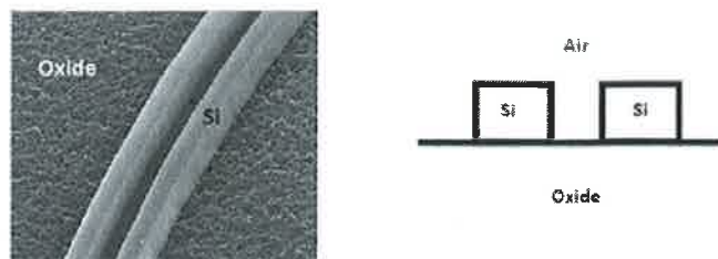
Figure 1: Top view (left) and cross-section of a slot waveguide (right).
